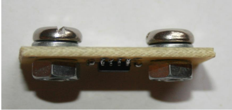
Fig. A-1. 6. PCB with electronics, screws, nuts, and washers (electronics on hidden surface)
