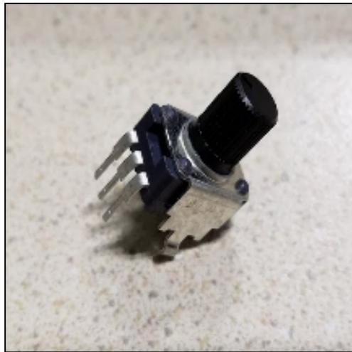
**Figure 12** Potentiometer used for Passive RoboPuppet angle sensing.
