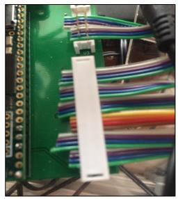
Figure 31 Wire Connection from Sensors to PCB.
