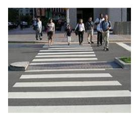
Figure 3: Standard Striped Crosswalk
