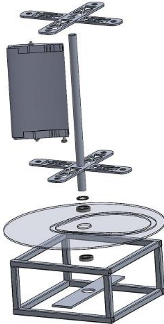
Figure 38: Exploded view of the mounting system
