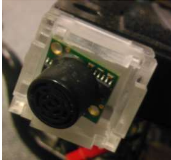
FIGURE 17: ULTRASONIC SENSOR WITH TOP KNOCKED OFF
