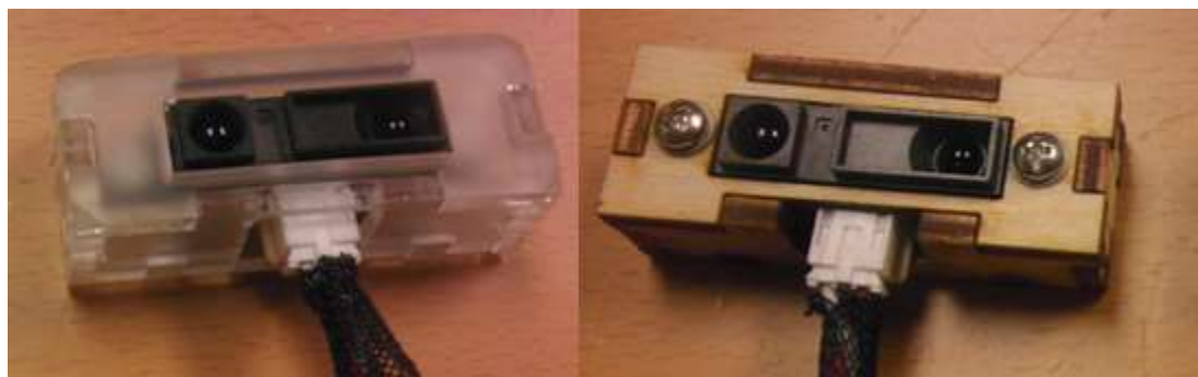
FIGURE 37: LEFT- OLD VERSION OF IR SENSOR CASING, RIGHT – NEW VERSION OF IR SENSOR CASING
