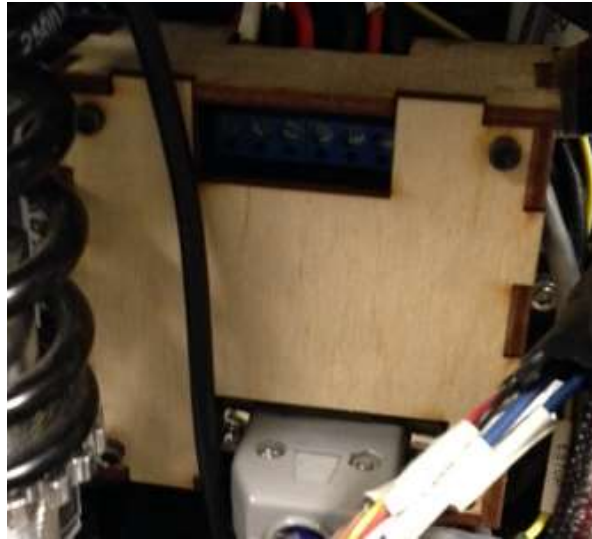
FIGURE 40: MOTOR CONTROLLER CASING MOUNTED ON WHEELCHAIR
