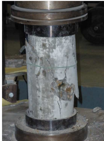
Figure 11: Compression failure in a fly ash concrete cylinder
