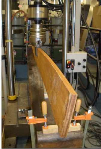
Figure 3: Lateral torsional buckling in an 1 ¾"x 11½" LVL beam
