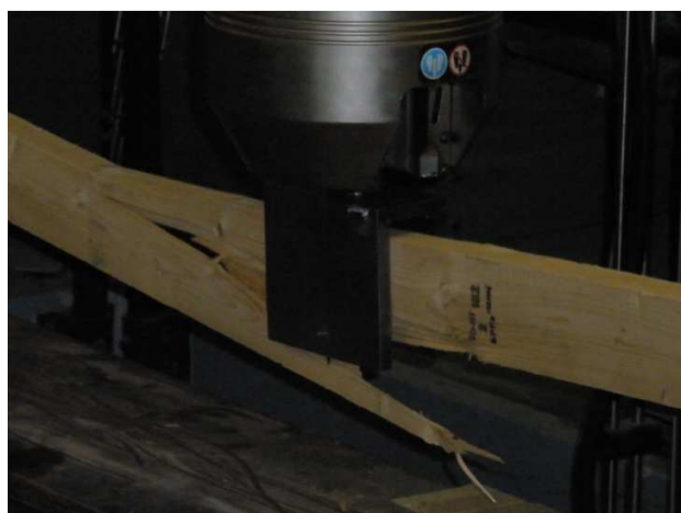
Figure 8: Typical bending failure in a Douglas fir 2"x 4" beam
