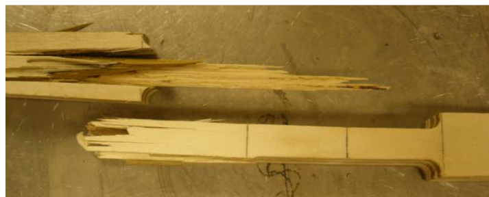
Figure 5: Typical failure pattern in an LVL tensile specimen
