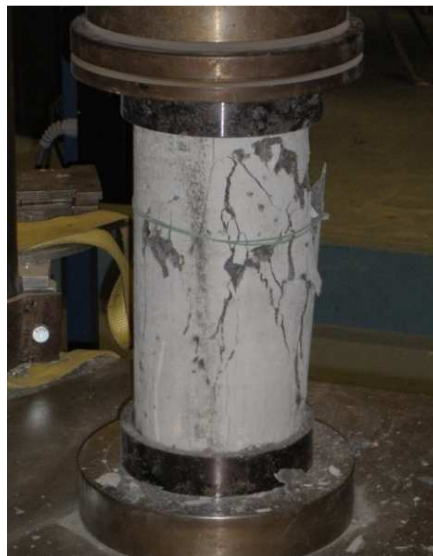
Figure 14: Compression failure in a silica fume concrete cylinder
