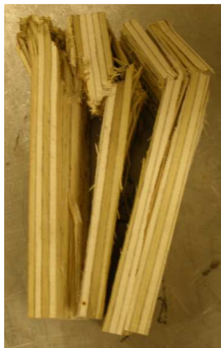
Figure 6: Typical failure in compression parallel to the grain of an LVL specimen
