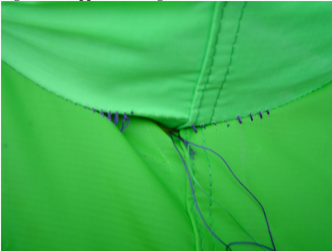
Figure 27: Ripped Stitching on Home Inflatable
