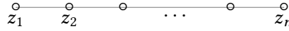
Figure 7.10: Discretization of the one-dimensional domain on which the finite element solution for the Helmholtz equation is described.
