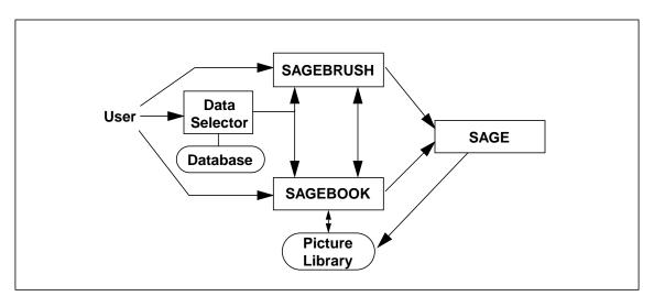
Figure 8: SAGE System Components
