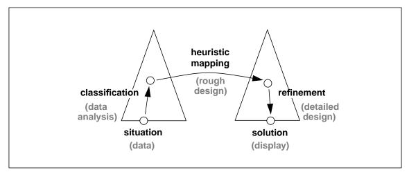
Figure 14: Rough and Detailed Design Seen as Classification
