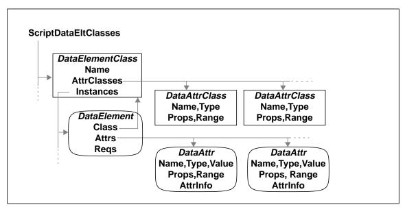
Figure 19: Data Element Storage Structure
