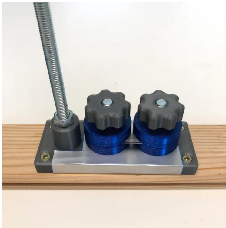
Figure 11: Existing bottle cutter updated design (Batek, 2023).
