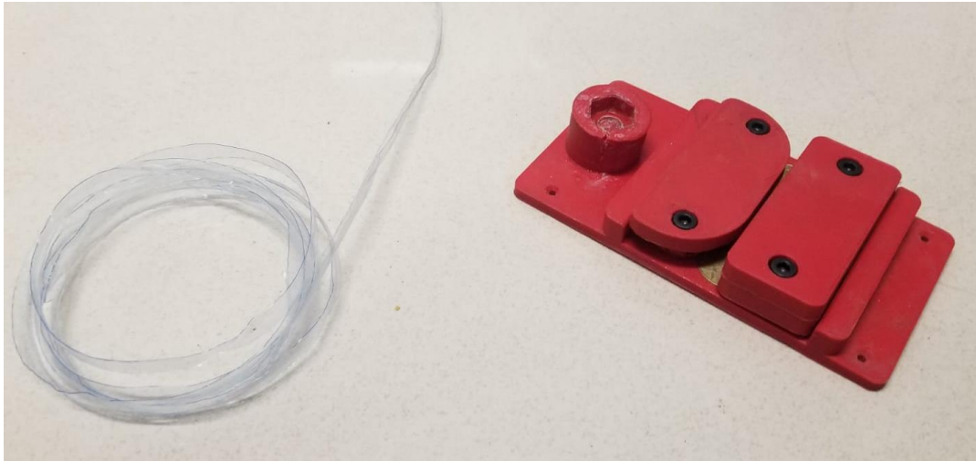
Figure 12: Rev. 1 of bottle cutter after destructive testing with spiralized bottle.
