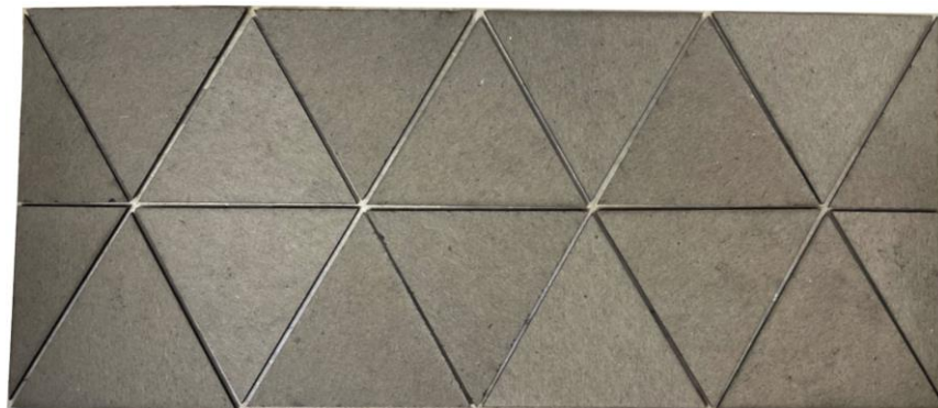
Figure 60. Wall made with 5-inch side length equilateral triangle
