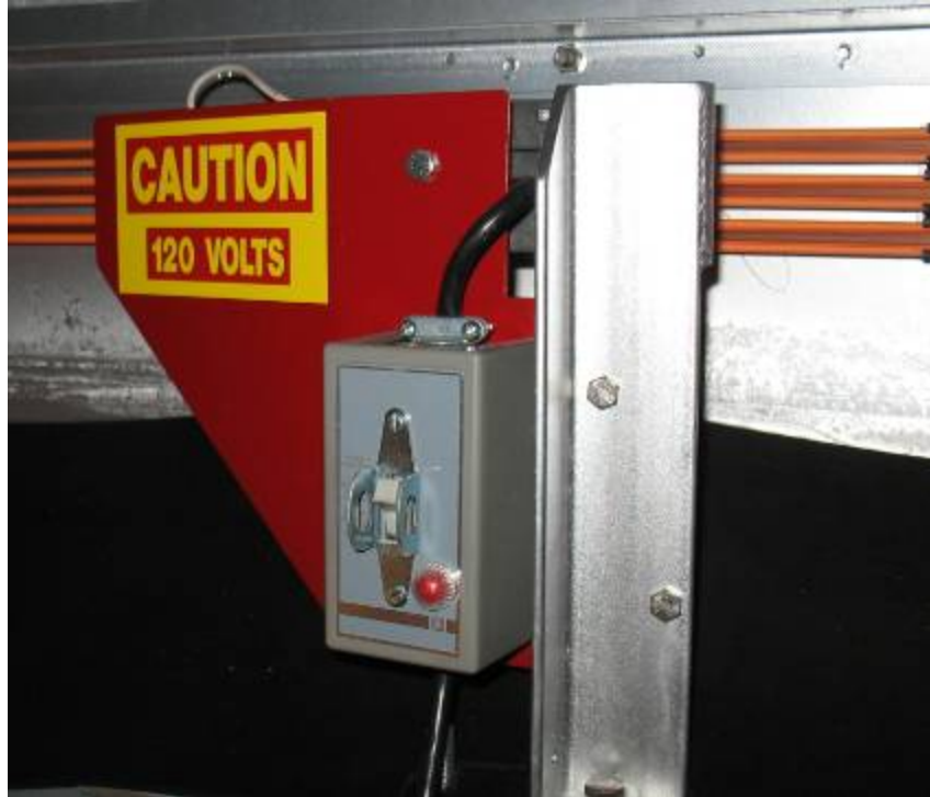
Figure 18: Slip rings move against stationary power supply
