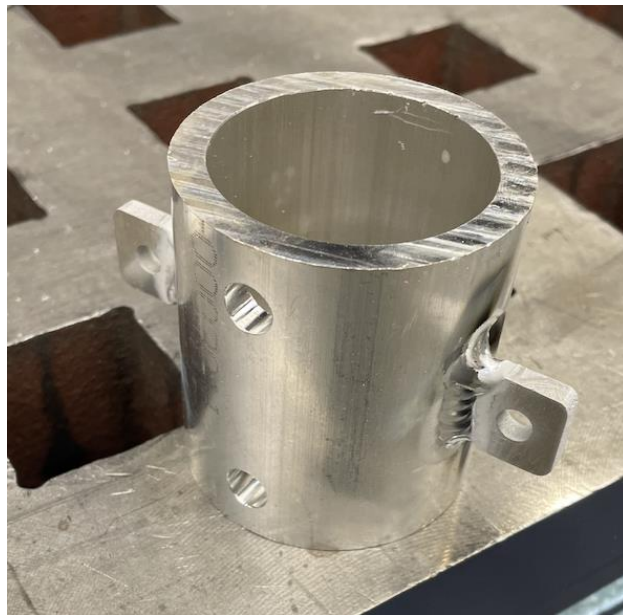
Fig. 30. A collar base half with the bolt wings welded on.
