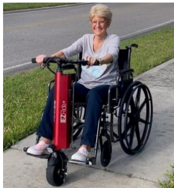
Fig. 6. Image of the EZRide power assist in use [3].
