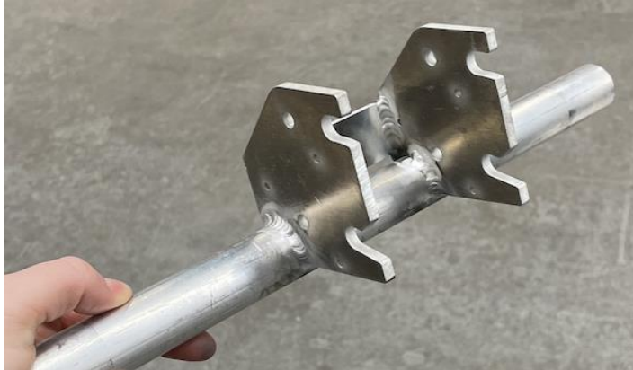
Fig. 29. Crossbar with the latch bottom welded on.
