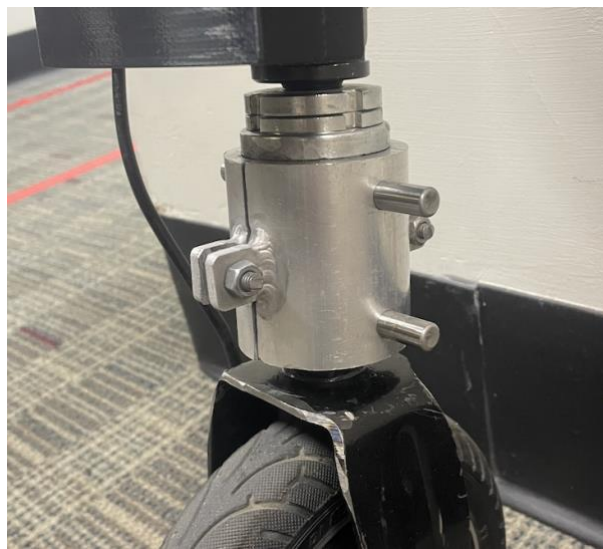
Fig. 32. Final collar assembly installed around the bearing box.
