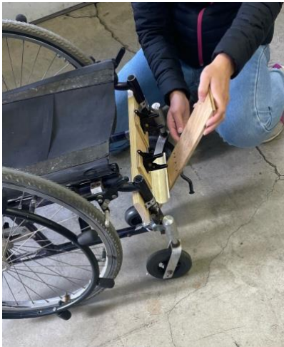
Fig. 15. Proof of concept of hook and gate latch design.
