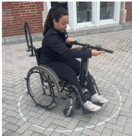
Fig. 33. Image of testing of the device turn radius.
