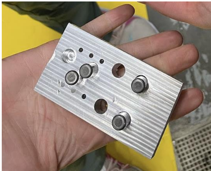
Fig. 27. Test piece for press fitting after testing.
