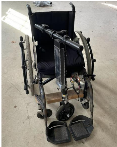
Fig. 11. Fixed proof of concept of the propulsion-aid.
