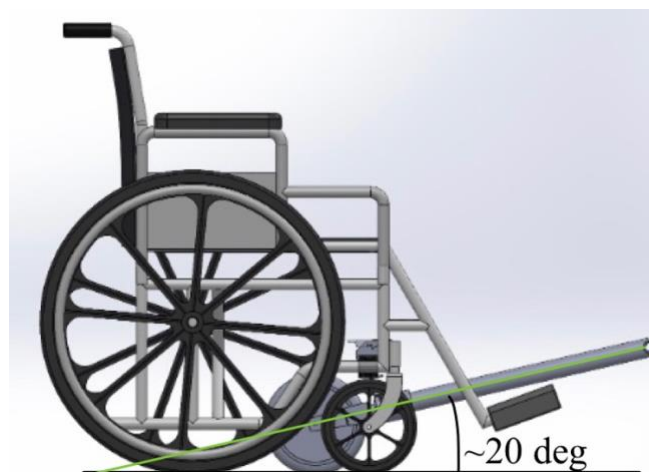
Fig. 18. CAD model showing the attachment angle with hook and gate latch design.
