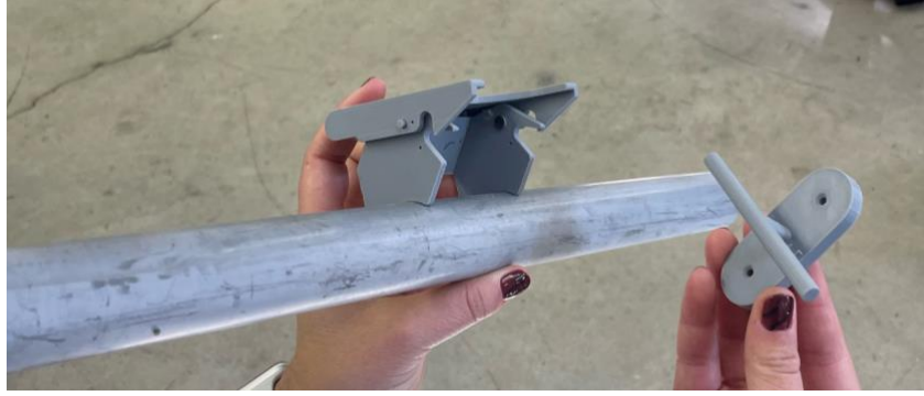
Fig. 16. First 3D print of the gate latch and hook design.
