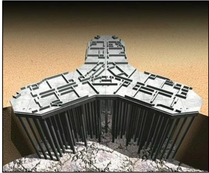
Figure 2.3.6. The Burj Khalifa's foundation. Concrete pilings go deep into the sand to keep the structure stable. 20
