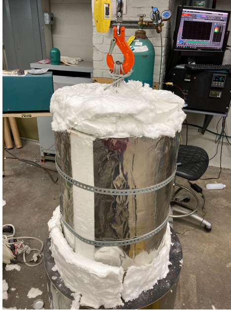
Figure 5.9: Secondary insulation elements wrapped in steel foil and tightened with 2 steel straphangers. Secondary insulation resting atop furnace.
