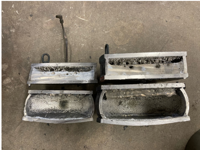
Figure 5.10: Cut 1-effect distiller after distillation showing the evaporated Mg in the Condenser
