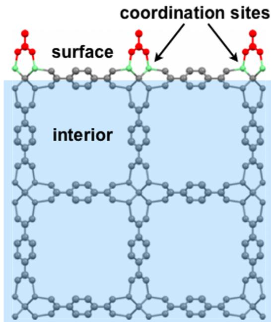
*Figure 1: Coordination of capping reagents onto the metal ions of MOF-5. The red molecules indicate the coordination sites to which capping reagents will orthogonally bind and trap molecules.<sup>5</sup>*
