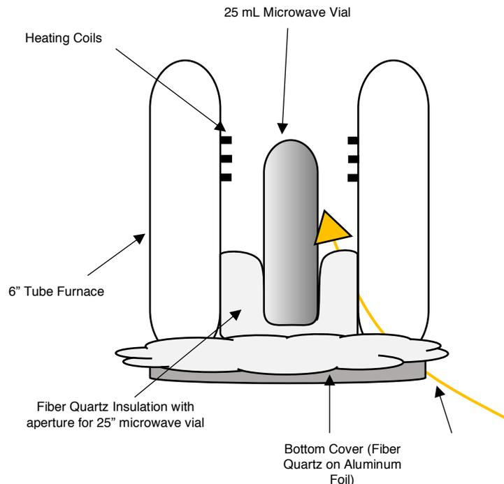
Figure 16: Schematic of tube furnace used to synthesize MOFs (interior view).
