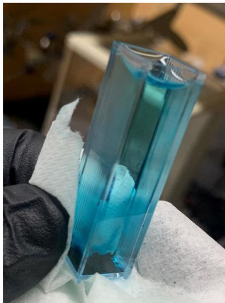
Figure 11: Image of MB loaded MOF-5 in ethanol with dye leaching out into solution, turning it blue.
