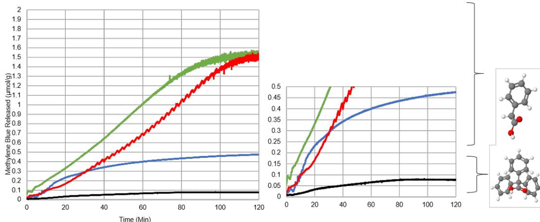
Figure 10 Results of Dye Release tests with MB in MOF-5 capped by PAA and TPAA. MOF-5 capped with TPAA leaches out minimal MB. MOF-5 capped with PAA leaches out significant MB.
