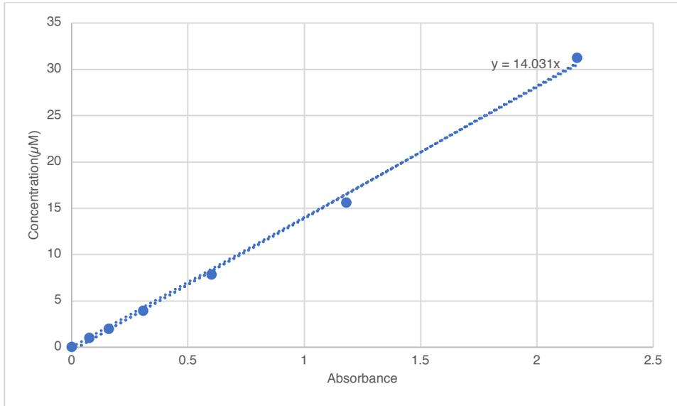
Figure 9: Calibration Curve for the quantification of MB leakage from MOF-5. The equation shown is that which outputs concentration (Y) based on the observed absorbance (X).
