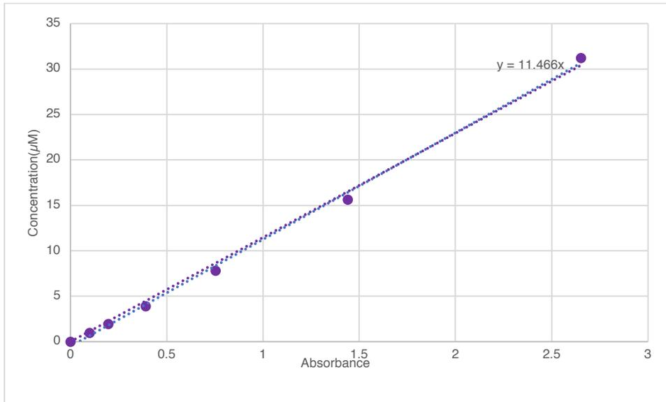
Figure 8: Calibration Curve for the quantification of CV leakage from MOF-5. The equation shown is that which outputs concentration (Y) based on the observed absorbance (X).
