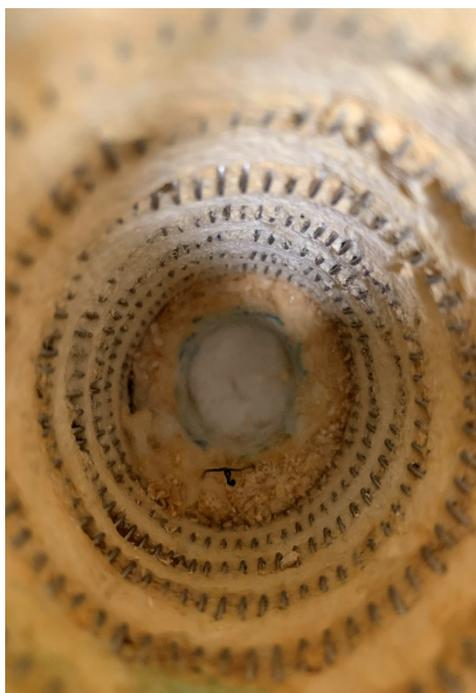
Figure 19: Interior view of the furnace with heating coils and quartz fiber molded vial slot in view. Thermocouple can be seen protruding from the bottom of the setup.
