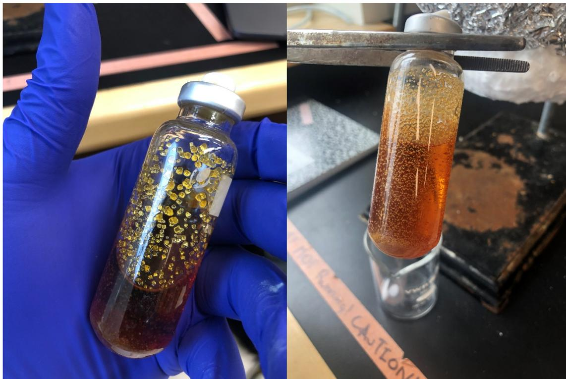
Figure 12: MOF-5 synthesized following the adjustment to the synthesis procedure. (Left) MOF-5 made by the previously established synthesis procedure.
