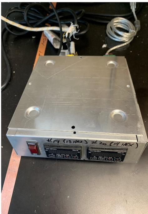
Figure 17: Love Controls model 32B-23 Temperature Process Controller
