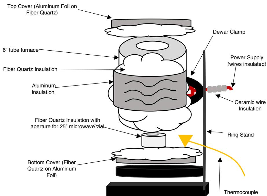
Figure 15: Schematic of tube furnace used to synthesize MOFs (exterior view).
