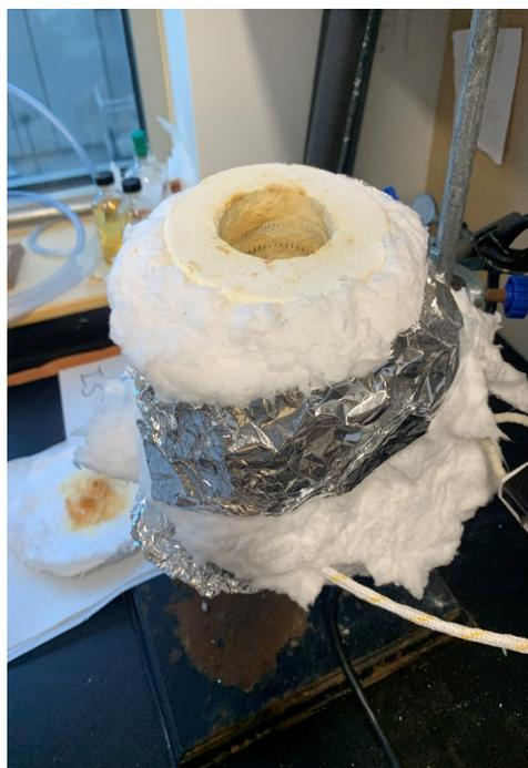
Figure 18: Top view of the MOF-5 furnace with aperture, braided thermocouple, quartz fiber with aperture, aluminum foil and ring stand in view.
