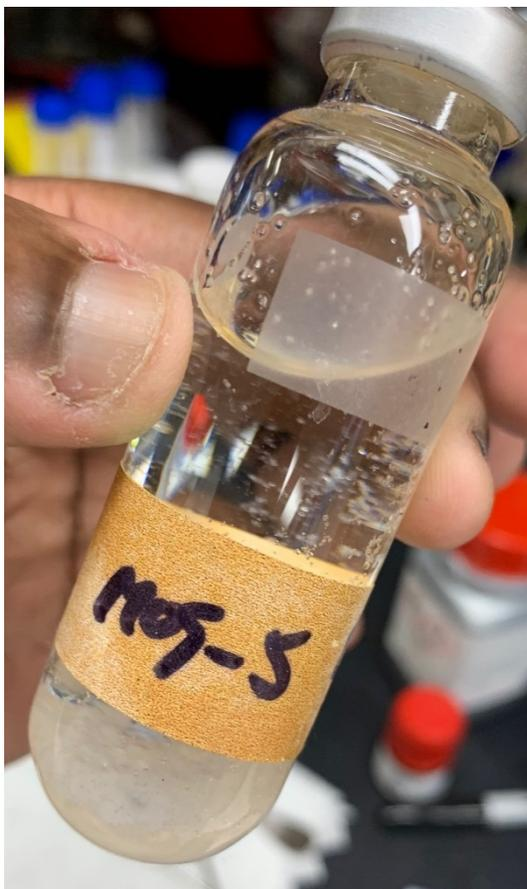
Figure 13: MOF-5 synthesized in DMF in solution.
