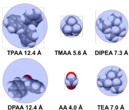
Figure 2: Relative sizes of capping reagents with Van der Waals radii. The size of these molecules largest to smallest is TPAA, DPAA, DIPEA, TEA, TMAA, and AA. Note that PAA was used but not reported and would go directly after DPAA in size.<sup>5</sup>
