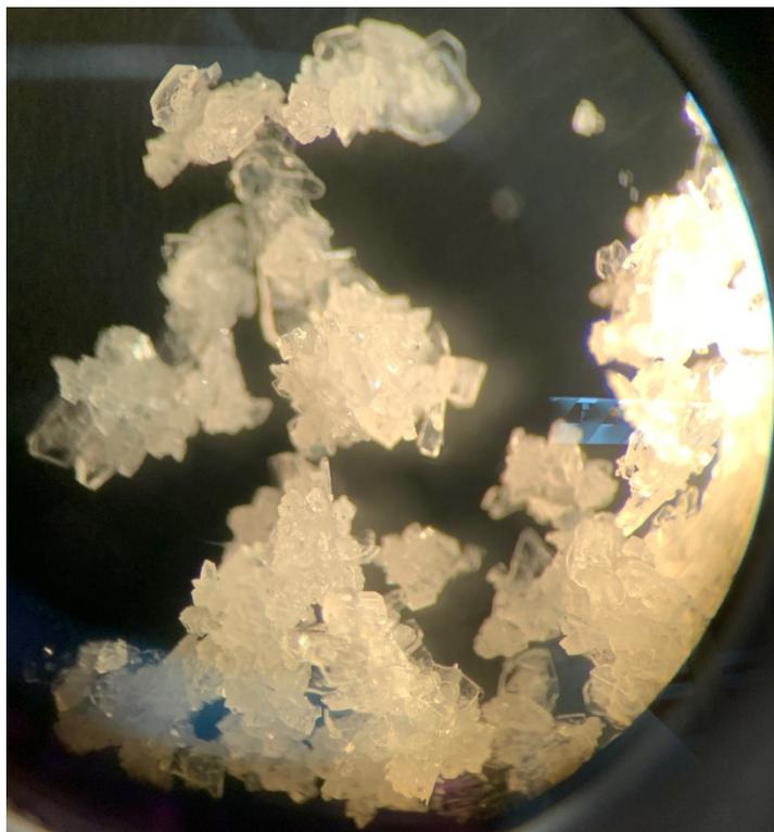
Figure 7: Microscope enhanced image of MOF-5 synthesized in DMF. The crystals are clear and white but smaller and less defined than MOF-5 synthesized in DEF.
