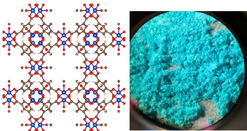
Figure 20: Schematic of HKUST-1 showing copper ions coordinated by benzene 1,3,5 tricarboxylic acid linkers (Left) Live image of HKUST-1 (Right).<sup>3-4</sup>
