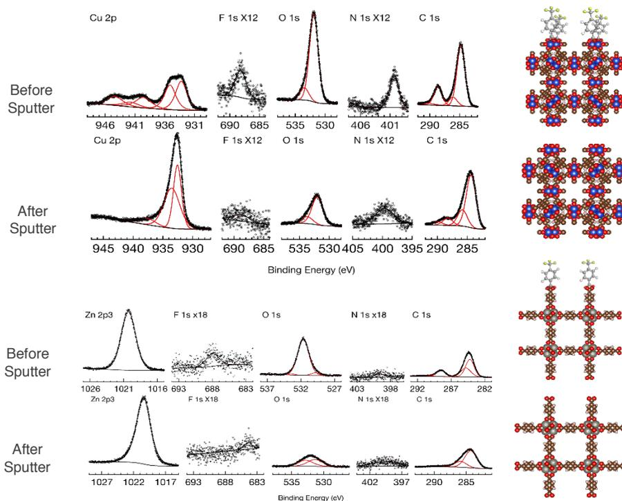
Figure 21: X-ray Photo Electron Spectroscopy results of capped vs. uncapped HKUST-1 and MOF-5. Sputtering shows the fluorinated groups situated on the surface of the MOFs as opposed to in the pores.<sup>2</sup>
