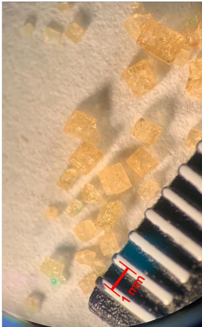
Figure 6: The size and appearance of MOF-5 synthesized in DEF. The crystals have a slight yellow tint and range in size from 0.5 to 1.5 mm.
