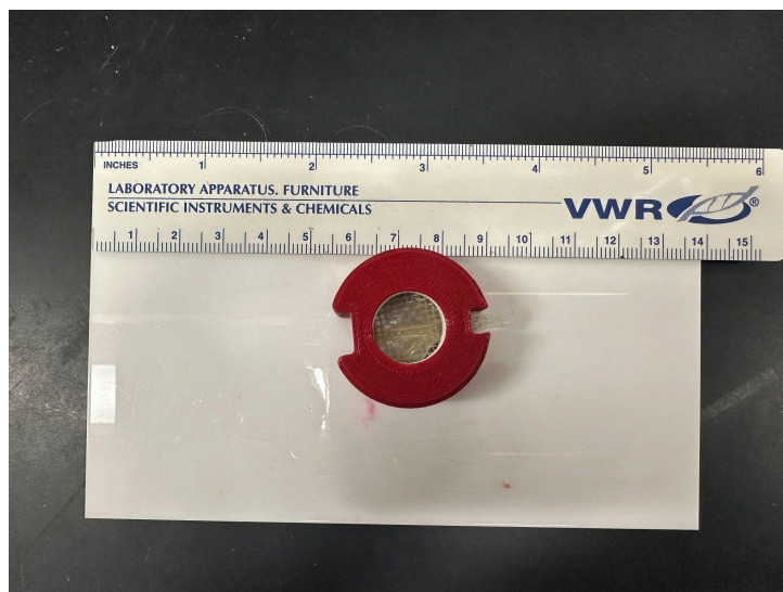
Figure 45: Shows the new housing device completely assembled with the decellularized leaf inside.
