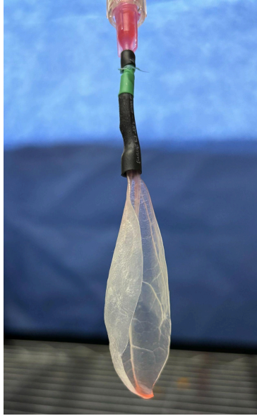
Figure 41: Shows image of the decellularized leaf attached to the gravity flow system before being perfused.
