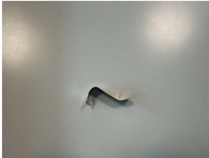
Figure 34: Image of the pry tool used to separate the bottom and top piece of the device.
