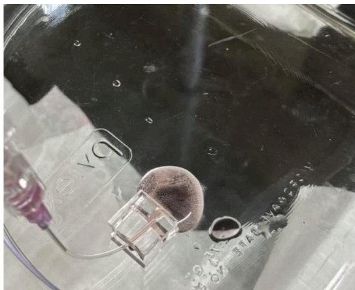
Figure 31: Perfusion of liquid through the multichannel PDMS microfluidic system through a cannula
