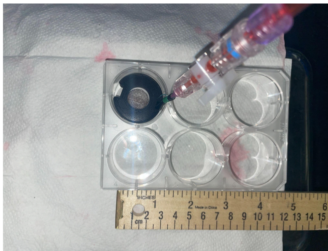
Figure 43: Image of the decellularized leaf before being perfused in the housing device.
