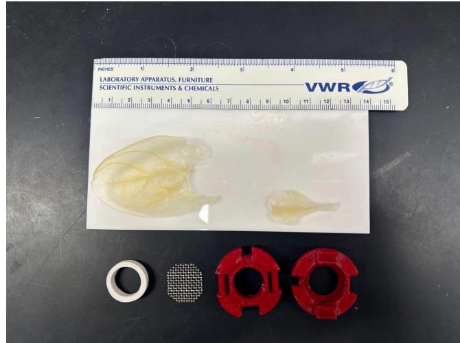
Figure 33: Image of the new housing device before being assembled with a decellularized leaf. There is a ruler for scaling purposes.
