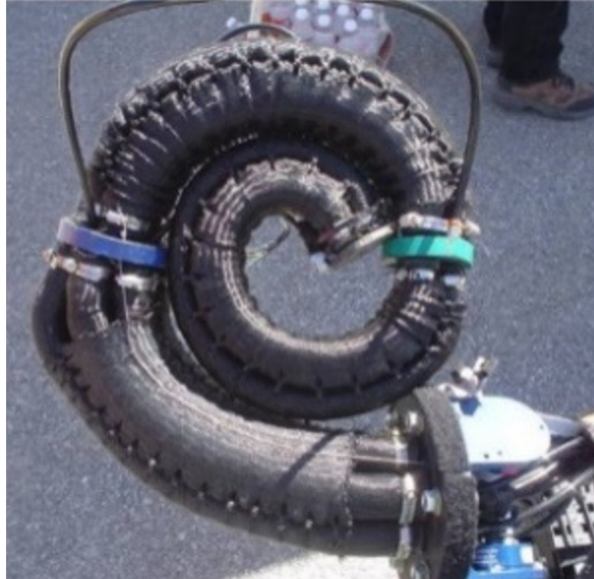
Figure 2.2: OctArm V-Continuum manipulator [2]
