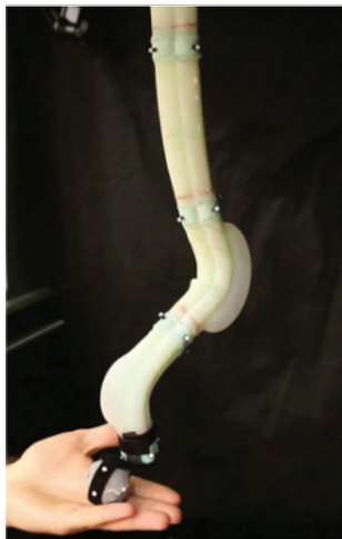
Figure 2.4: Soft fluidic elastomer manipulator gently taking a small ball from the palm of its human collaborator. [4]
