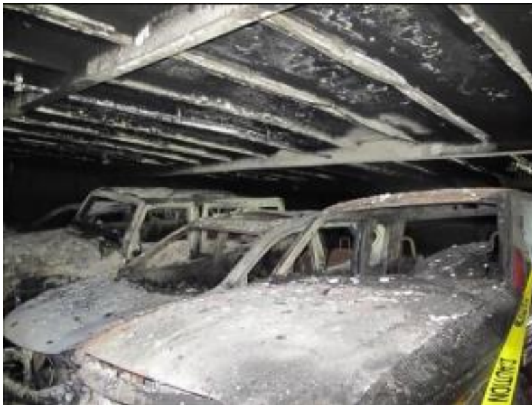
Figure 13. Burnt vehicles on the vessel Honor, showing the close packing of the cars. By the National Transportation Safety Board, 2017, image is in the public domain.
