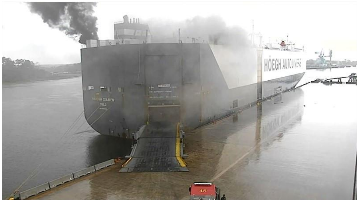
Figure 9. Smoke coming from aft cargo deck ventilation housing exhausts on Höegh Xiamen. By National Transportation Safety Board, 2021, image is in the public domain.
