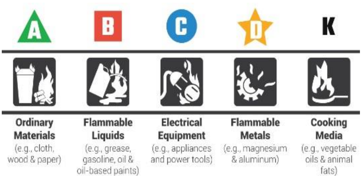
Figure 24. A sign detailing the classifications of fires determined by the NFPA for assistance in choosing an adequate extinguisher for a given fire. By the City of San Jose, n.d., image is in the public domain.
