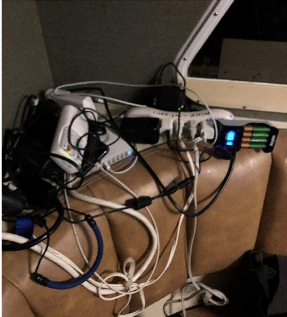
Figure 10. Photo taken during accident voyage of MV Conception showing overcharging onboard. By J. Dignam and National Transportation Safety Board, 2019 image is in the public domain.
