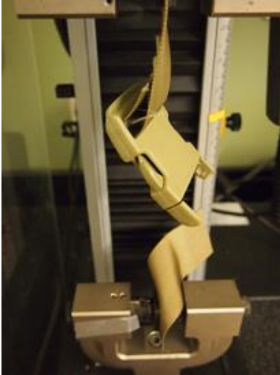
Figure 28: Failure of Side Release Buckle
