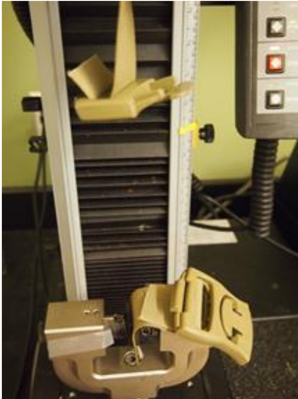
Figure 29: Failure of Center Release Buckle
