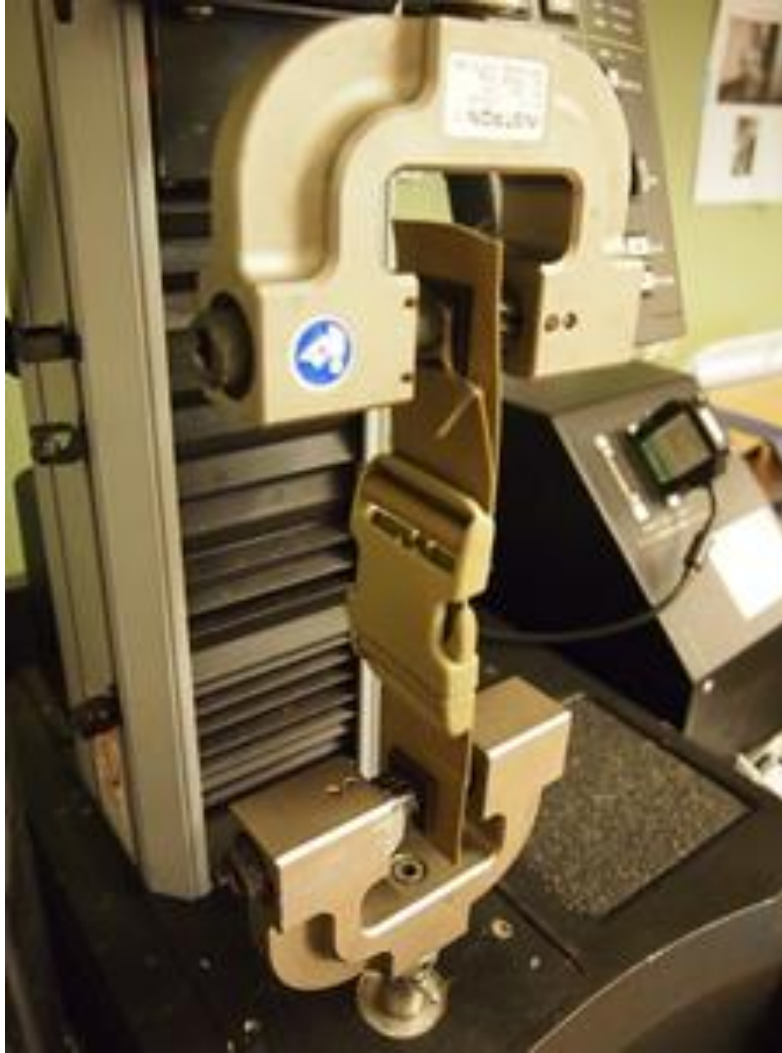
Figure 27: Tension Testing Setup
