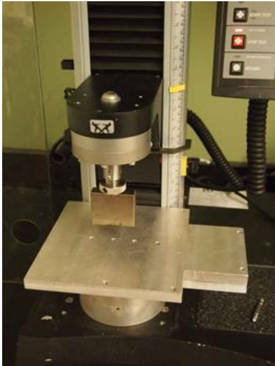
Figure 25: Compression Testing Setup
