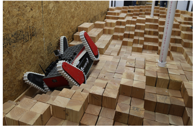
Figure 88: The WALRUS Rover traversing a NIST Symmetric Stepfield
