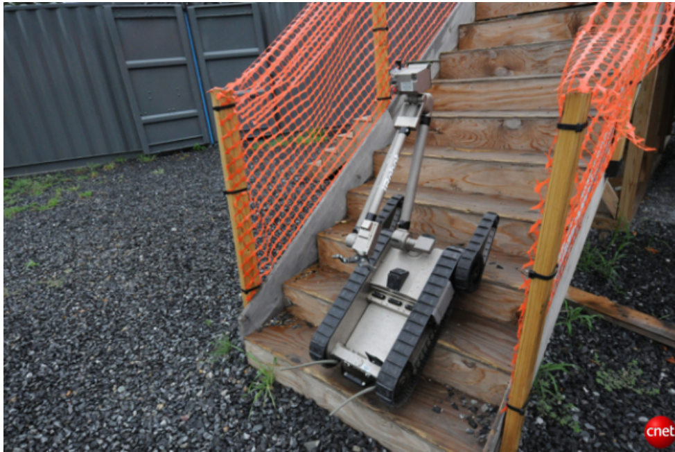
Figure 3: PackBot using its arm forward to change its CoG.[15]
