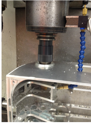
Figure 28: Post-processing the chassis
