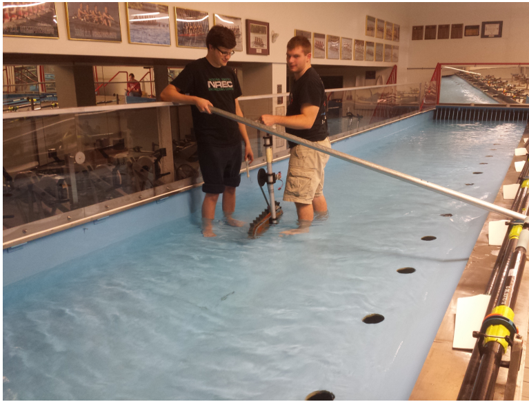
Figure 26: Thrust testing in the WPI Rowing Tanks.
