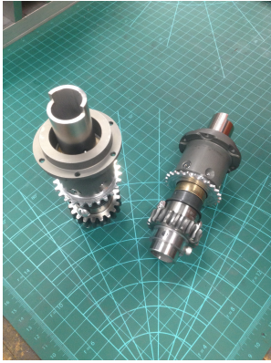
Figure 27: Inline Drives during assembly
