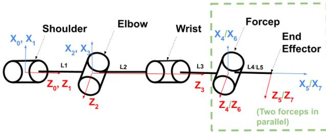
Fig. 2 Kinematic diagram of the instrument.
