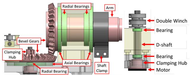
Fig. 4 Side views of shoulder (left) and driving shafts (right)
