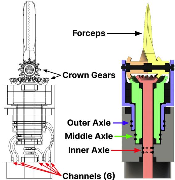
Fig. 8 Wireframe side view (left) and cross section front view (right) of wrist roll and forceps.
