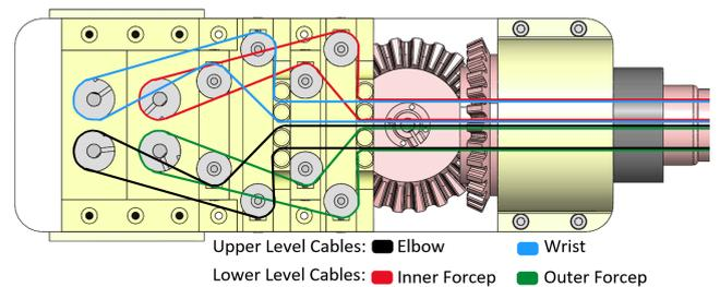
Fig. 5 Cable paths on base plate.
