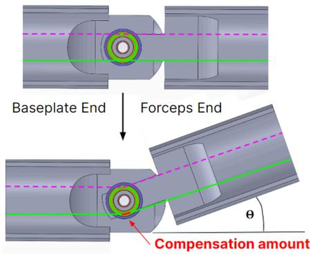
Fig. 10 Visual representation of cable length compensation in the elbow joint.
