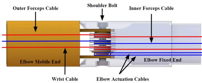
Fig. 6 Elbow top down view with transparent fixed end. Pulleys in the center for organization of the cables needed to actuate the wrist and forceps.
