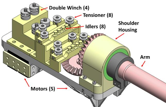
Fig. 3 Isometric view of base plate.
