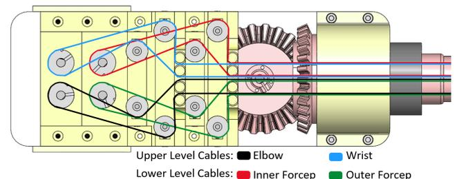
Fig. 5 Cable paths on base plate.
