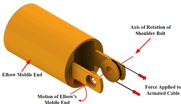
Fig. 7 isometric view of the mobile end of the elbow.
