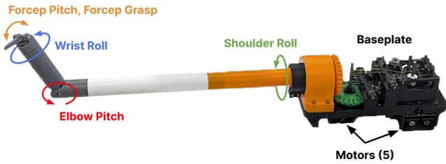
Fig. 1 Five DoFs instrument prototype with its unique kinematic layout that includes both shoulder and wrist roll.
