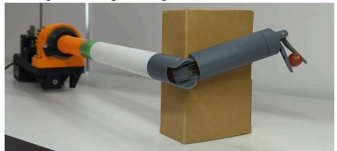
Fig. 13 Device manipulating a grape behind an obstacle.
