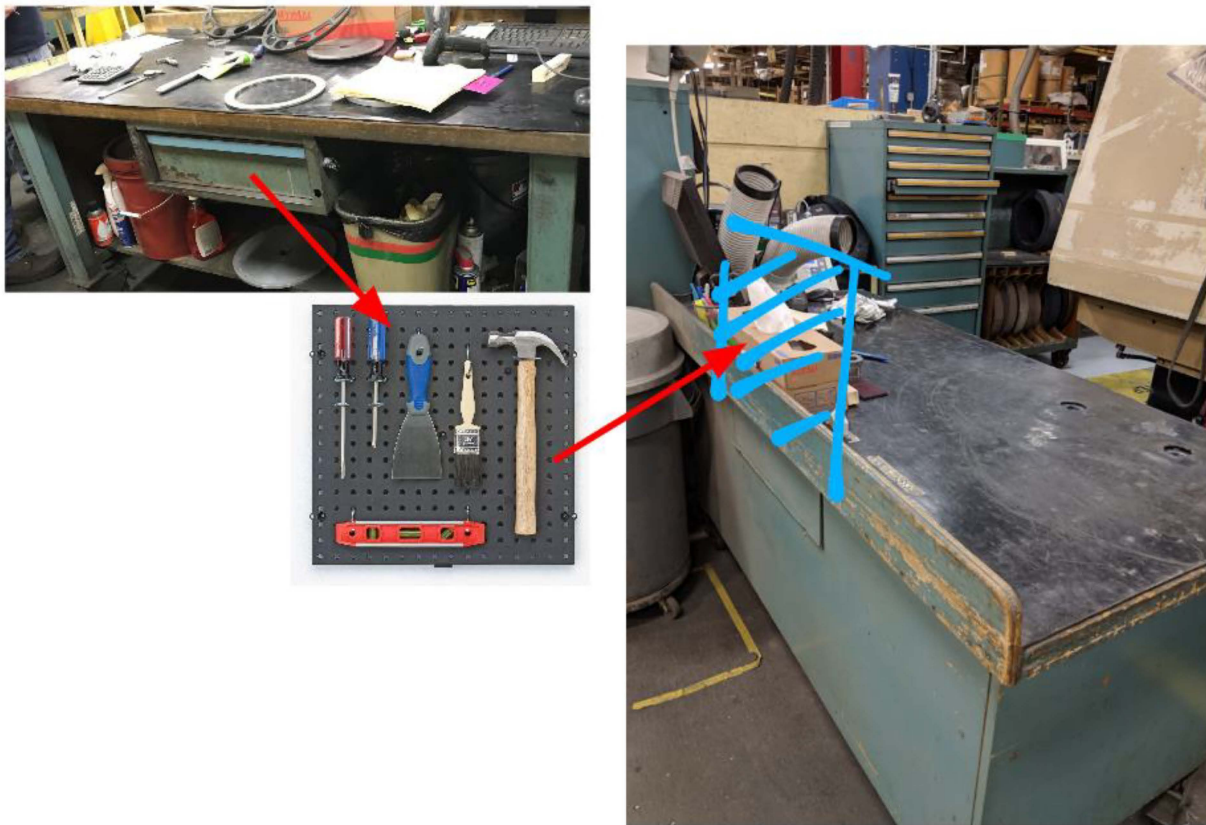
Figure 10. Proposed relocation of commonly used tools in the OD grinding machine area.
