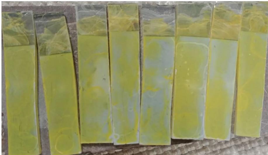
Figure 25: Post annealed SnO 2 /BiVO 4 electrodes synthesized using drop-coating
