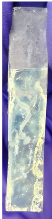
Spray Coating (2) (2-layer 0.05 M)
