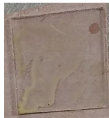
Figure 21: Cell with 1 layer of \text{WO}_3 using drop-coating method. 50 mL of 0.02 M solution dropped onto 2.5 x 2.5cm glass annealed at 500°C for 2 hours ramping for 4 hours.
