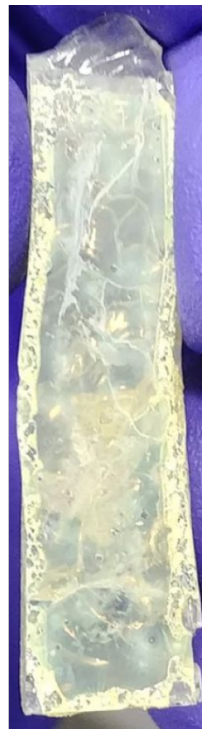
Spray Coating (2) (3-layer 0.05 M)
