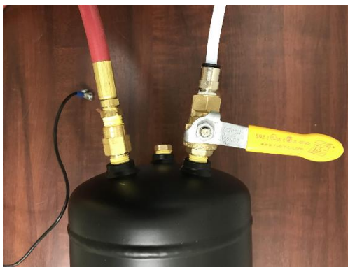
Figure 5A: Yellow valve handle perpendicular to air tank in the closed position
