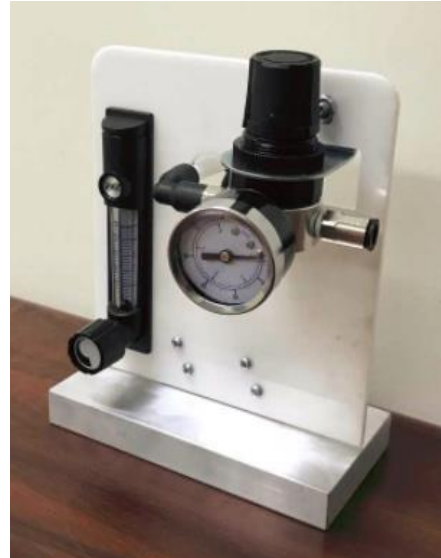
Figure 7B: Fully assembled airflow regulation unit
