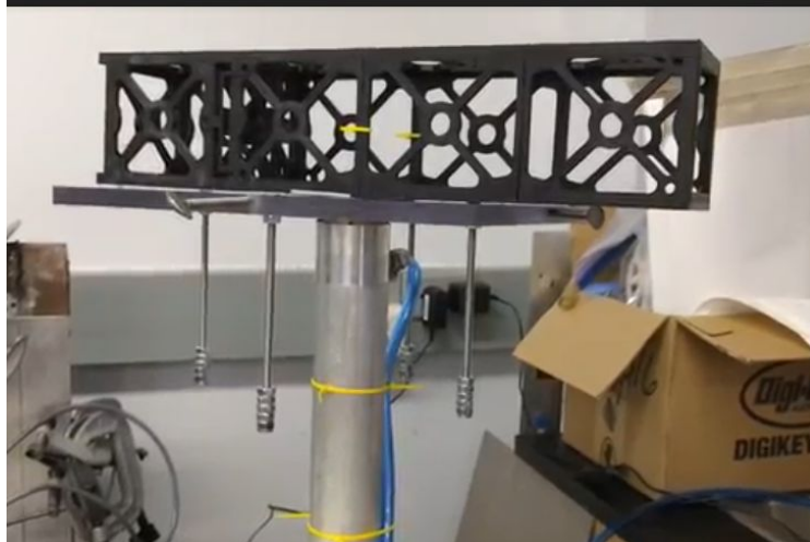
Figure 6.1. Prototype CubeSat and Test bed at Equilibrium.
