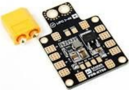
Figure 5.14. Power Distribution Board[33]
