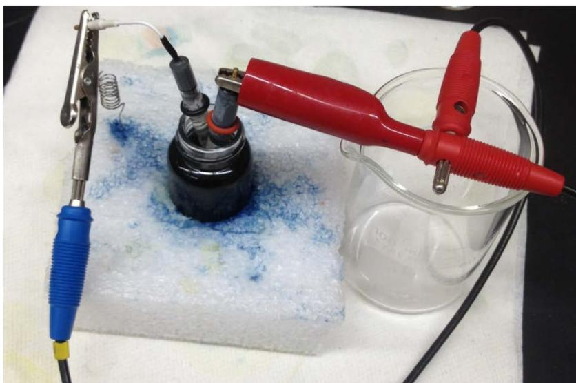
Figure 33: Setting up the biosensor for PPy deposition
