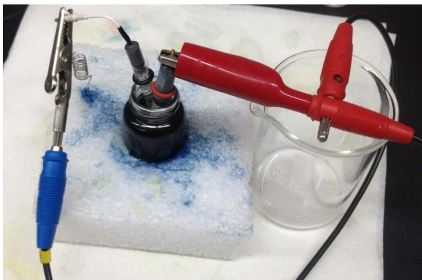
**Figure 25: PPy electrochemical film deposition set up**
