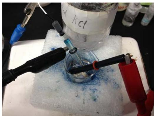
Figure 26: Set up of the lactate amperometry
