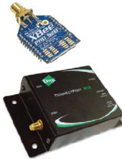
Figure 3: SolarEdge Zigbee-Ethernet Gateway
