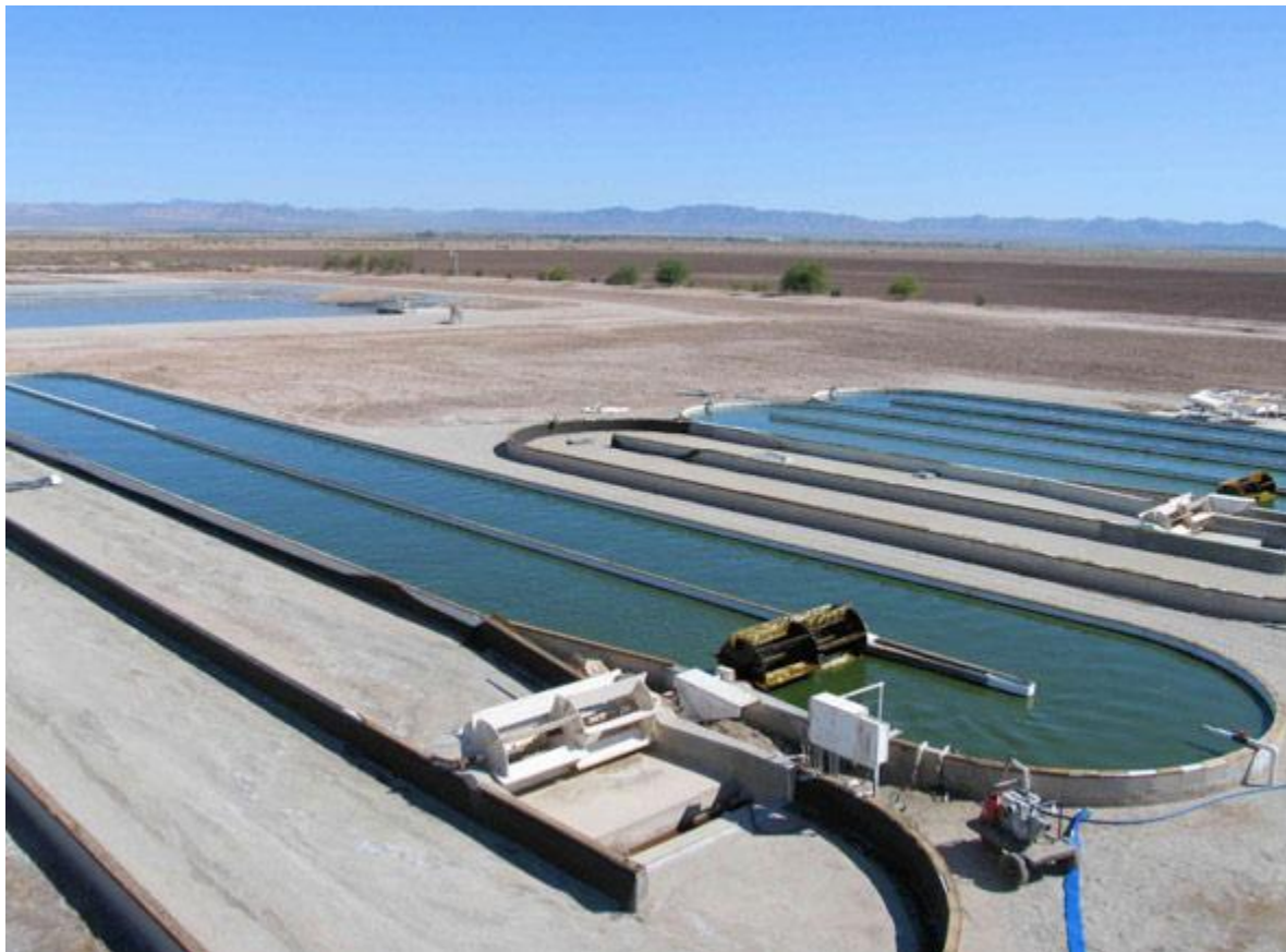
Figure 6: Picture of a few of the 11 ponds located in the California's Imperial Valley, each containing more than 200,000 gallons of water. [24]
