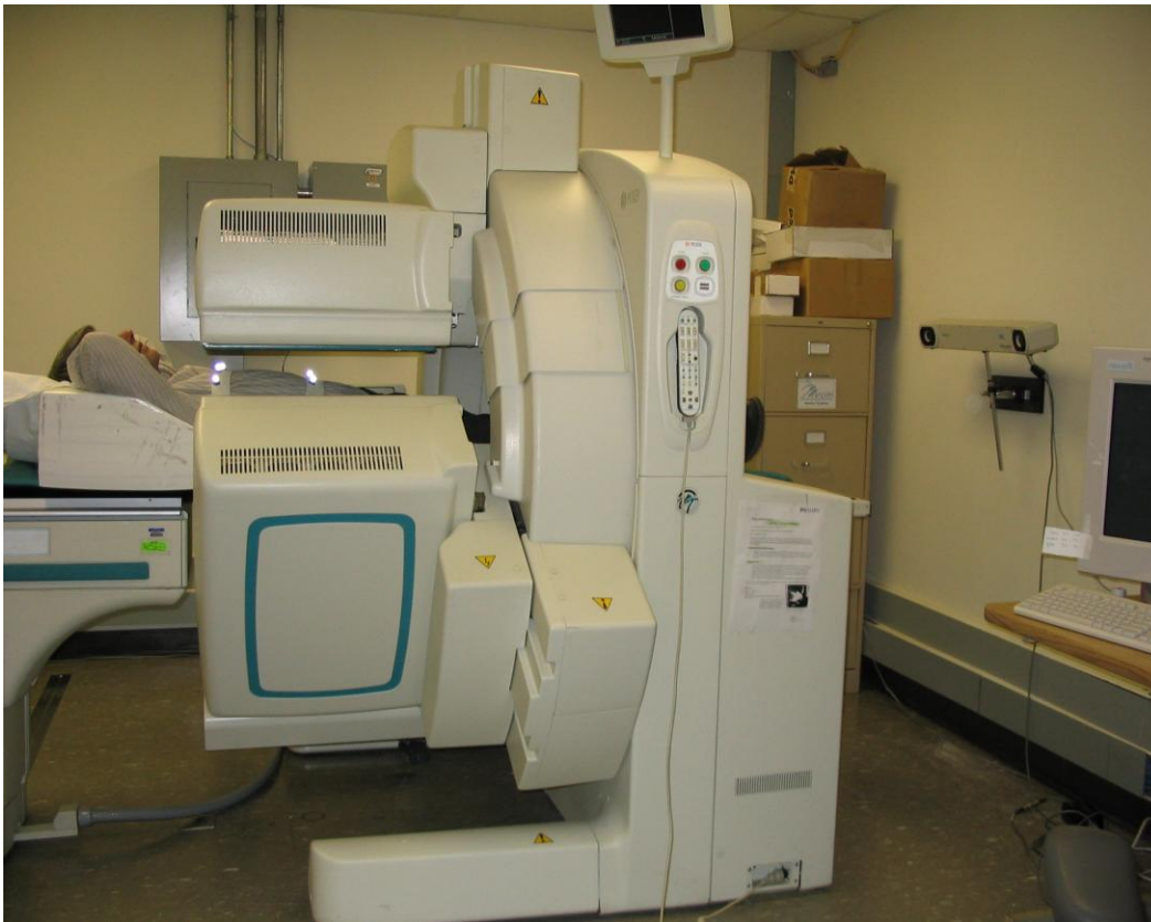
Fig. 1. The Polaris system is seen on the far right mounted on the wall. It views the Infrared (IR) reflecting spheres (white spots) on the anterior surface of patients on two elastic belts. The upper chest belt, by our chosen convention, contains markers 1 through 4, starting with 1 on the patient's right. Similarly, the lower abdomen belt has markers 5 through 8, starting with 5 on the patient's right.
