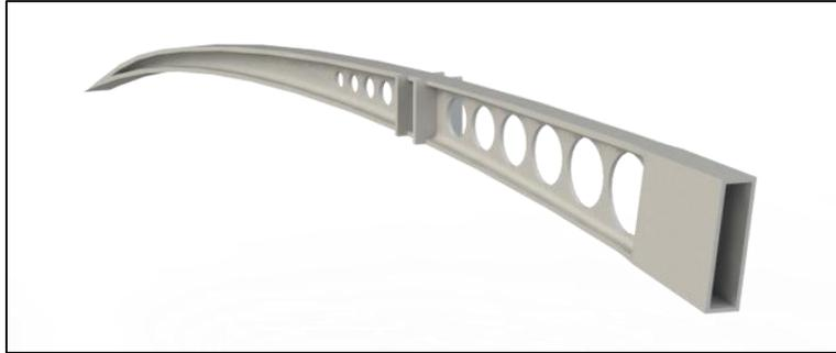
**Figure 14: Typical Trailing Edge Rib**
