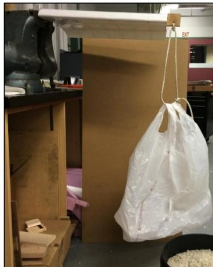
**Figure 71: Inner Wing Structural Test Setup**
