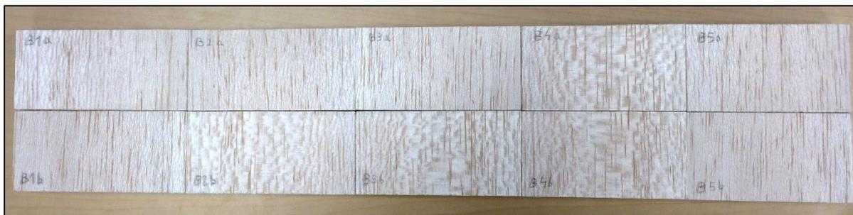
**Figure 75: B-Section Spar Webs Ready for Assembly**
