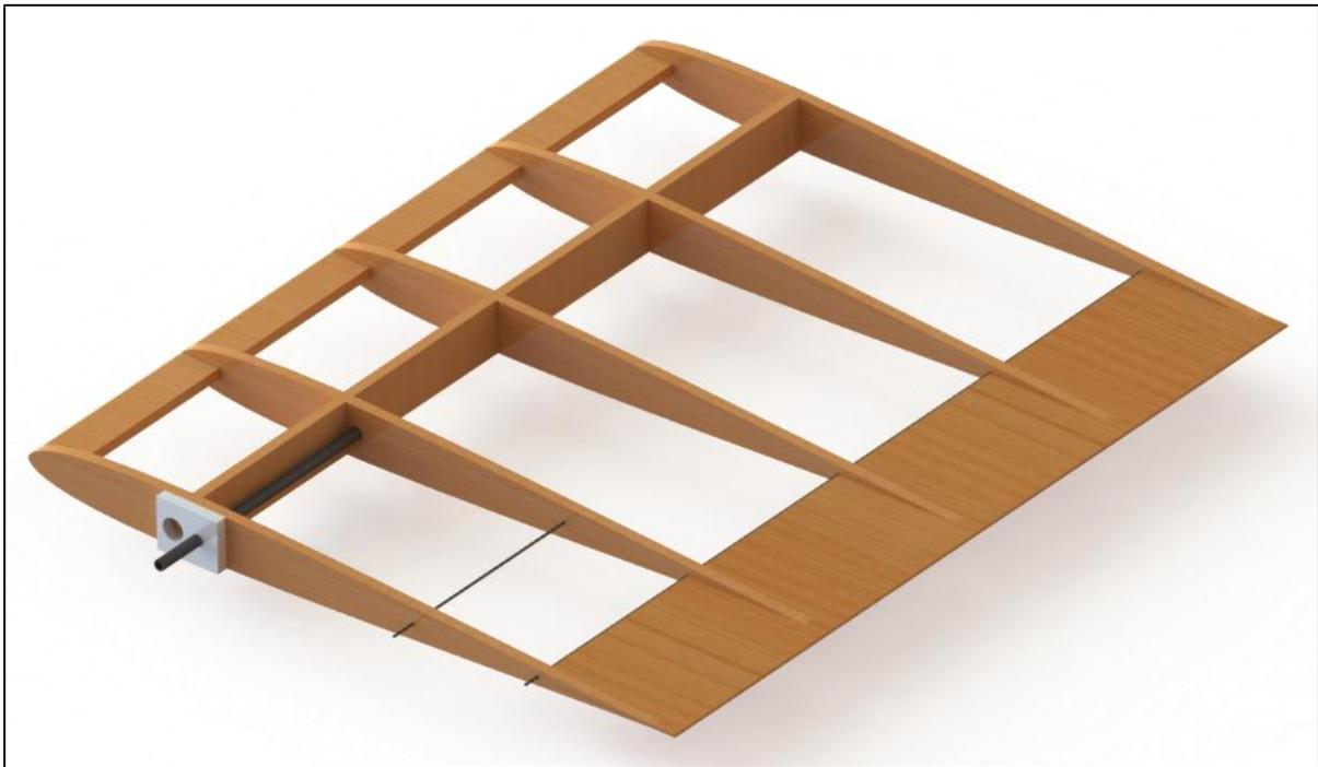
**Figure 35: Vertical Stabilizer Structure**
