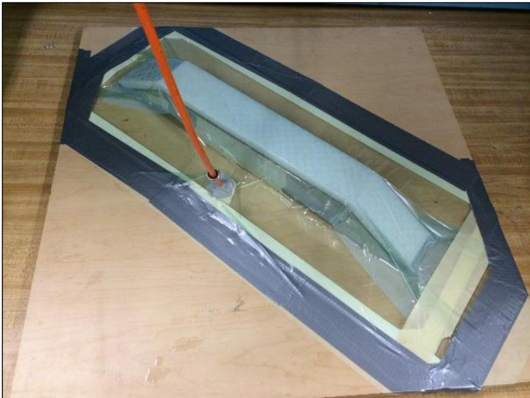
Figure 79: Landing Skid Vacuum Lamination
