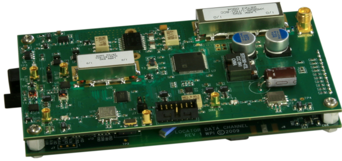
Figure 2.7: Revision 2 PCB Stack (RF Hardware on Top, Data Channel Underneath)
