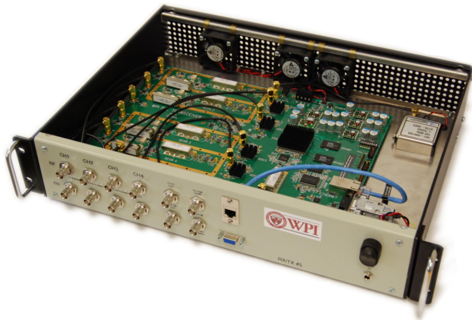
Figure 2.9: Revision 2 Reference Hardware – The Transceiver Box
