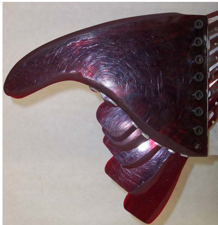
Figure 16. Test Wing in with Feathers Fully Retracted
