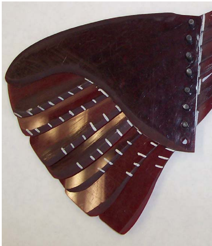
Figure 15. Test Wing with Feathers Fully Extended for Zimmerman Representation
