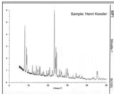
Figure 13: XRD of Silicalite-1 Crystals from the IZA Website
