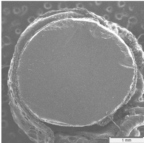
Cross Section of Bead at 20X
