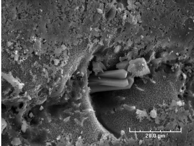
Bead with Silica:TPA ratio of 5.6 at 2,000X
