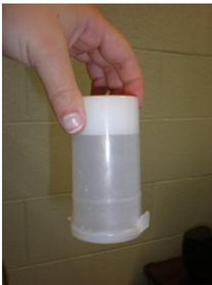
Figure 21: Solution Aged One Week at Room Temperature Turned Upside Down
