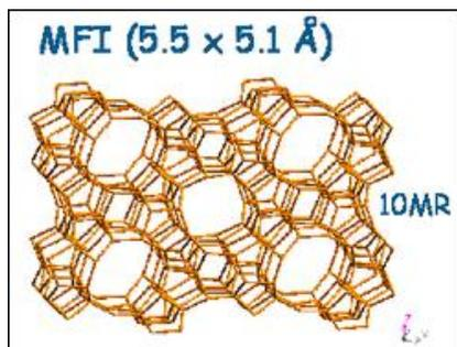
Figure 1: The MFI Structure.<sup>1</sup>
