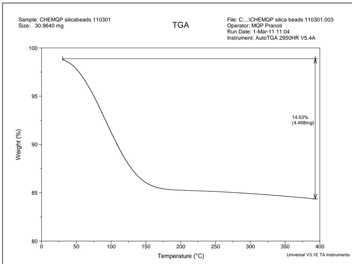
Figure 14: Results from TGA Analysis of a Silica Bead
