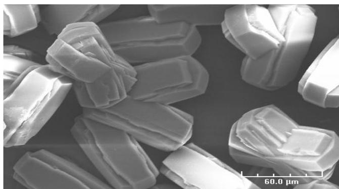
Figure 22: Twinning and intergrowths from aged solutions; heated 7 days at 150 °C
