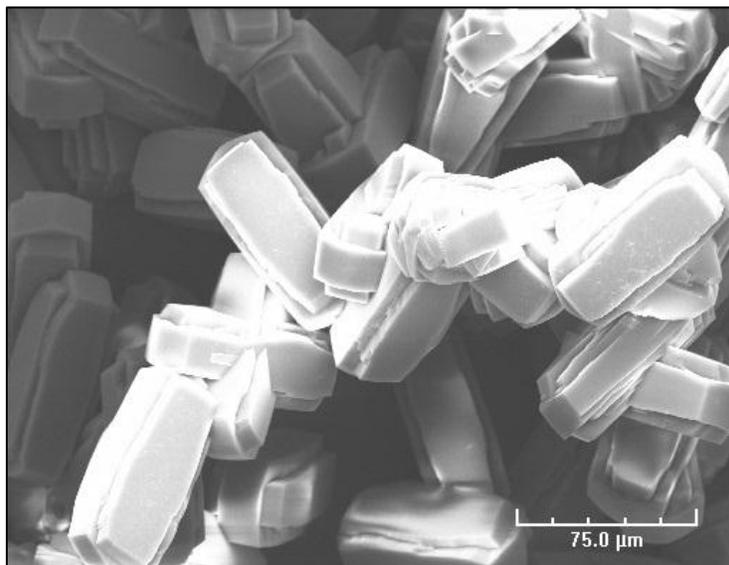
**Figure 11: Silicalite-1 Crystals Made Using Sylvie Gonthier's Batch Composition, Image at 500X**
