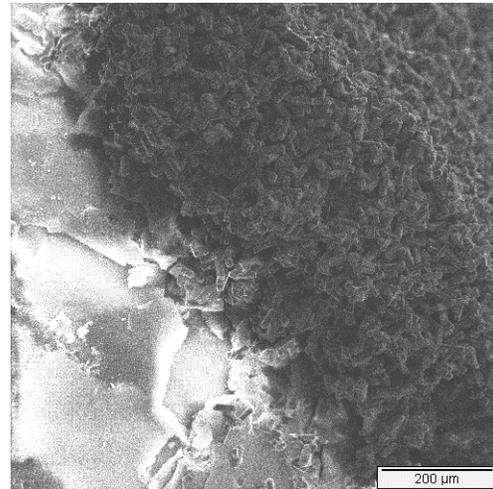
Figure 35: Crystals on the Outer Surface at 100X
