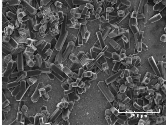
Figure 23: The outer surface of the bead with silica in the solution at 500X
