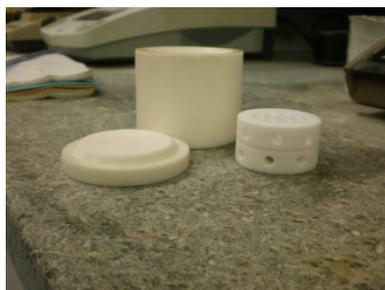
Figure 9: Teflon Lid, Liner, and Trays
