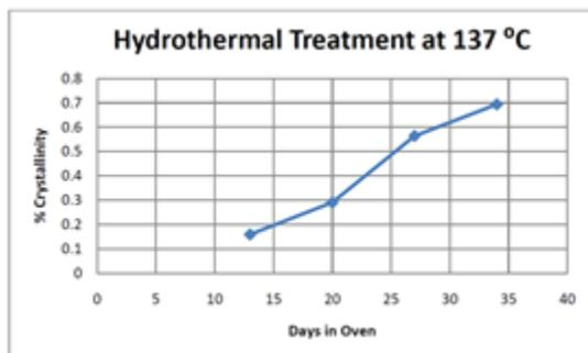
Figure 3: Percent Crystallinity vs. Days in Oven at 137 °C
