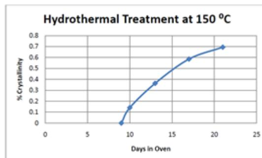
Figure 4: Percent Crystallinity vs. Days in Oven at 150 °C
