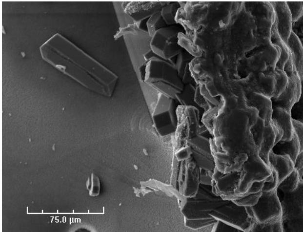
Cross Section of Top Bead at 500X
