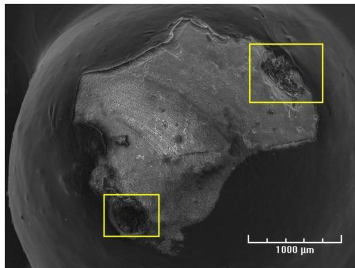
Figure 24: Two sections of crystal growth on the bead without silica solution at 40X
