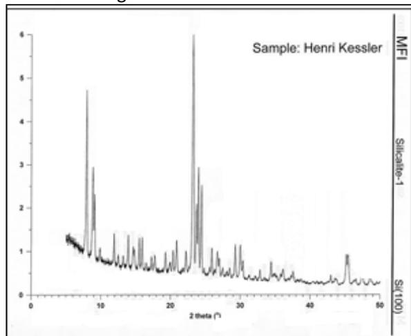
Figure 2: Typical XRD Pattern for Silicalite-1.<sup>10</sup>
