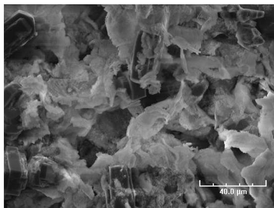
Figure 31: Aerogel Bead Powder at 700X
