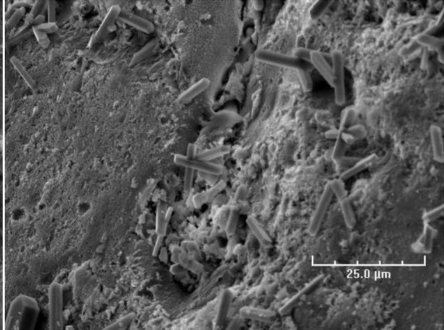
Bead with Silica:TPA ratio of 5.6 at 1,000X
