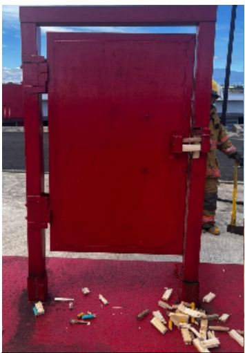
Figure 4: Forced Entry. This metal door is used to practice breaking a lock to enter a building with a Halligan bar.
