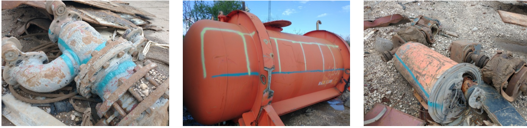
FIGURE 2.4: Three scrap pieces with desirable cutting paths on their surfaces painted by an experienced scrap cutting foreperson.
