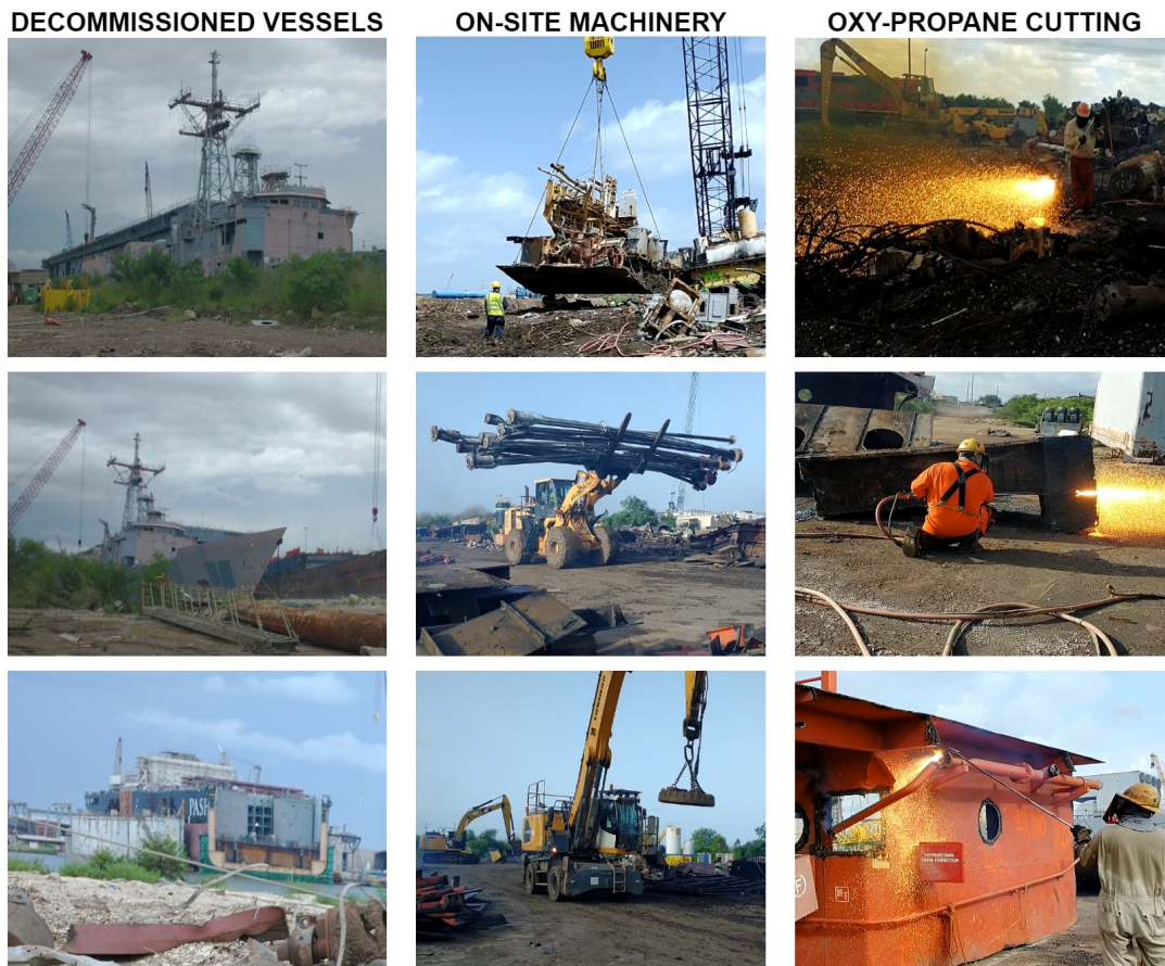
FIGURE 2.1: In the shipbreaking yard, the breakdown of decommissioned vessels is conducted via oxy-propane gas cutting and its ancillary logistics are facilitated using on-site machinery.
