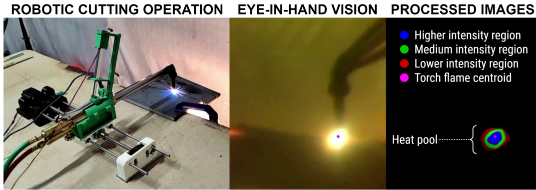
FIGURE 5.1: The proposed vision-based control algorithm enables the 1-DOF cutting robot to autonomously cut steel plates of different thicknesses. Left: Third-person view of the robot during control. Center: Eye-in-hand view of the metal surface showing the heat pool. Right: Processed stream of the eye-in-hand footage focusing on the shown heat pool. © IEEE
