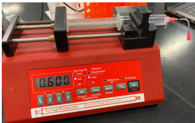
Figure 4.7. The New Era Pump System Inc. Syringe Pump from SyringePump.com (Model No. NE-300, Volts/Hz: 12V DC, Amperage: 0.75, Series No. 288793) is used to compress a 12mL syringe plunger at a steady rate. The syringe is connected to a 20g x 1/2" Luer stub adaptor, then a PVC tube, and another Luer stub adaptor. The second adaptor is attached to the needle reservoir, Figure 4.8. The inner diameter of the syringe and crosshead speed are set manually; therefore, these two values can be iterative.
