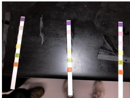
Figure 39. Aerobic, Final Settling, Final Effluent water test strips
