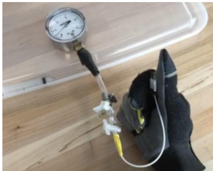
Figure 13: Black Glove Prototype with Analog Pressure Gauge
