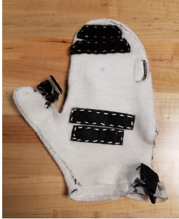
Figure 16: Modified White Glove Prototype for Pulse Monitoring
