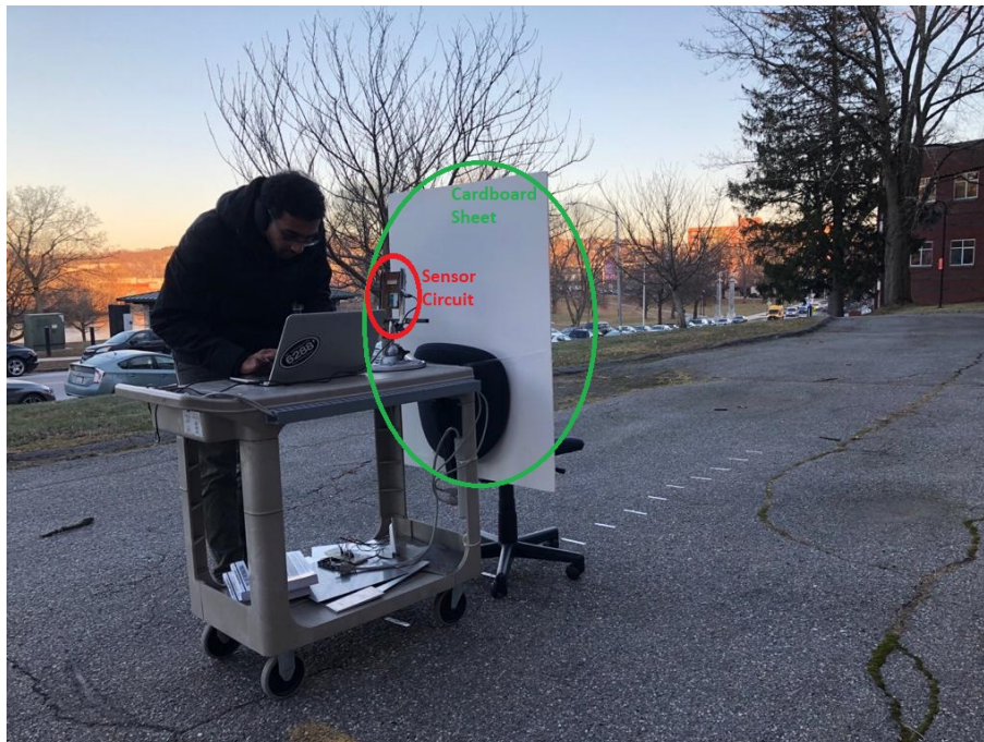
Figure 20: Testing MB1020 Ultrasonic sensors outdoors in an open driveway
