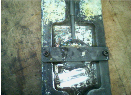
Figure 4.4b: Plastic Curing Inside of Casting Block
