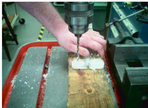
Figure 4.6a: Tapping Holes into the Mold Using the Drill Press
