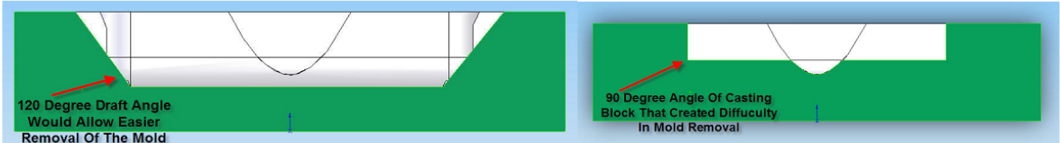
Figure 4.5b: Casting Block with Easier Release Angle Compared to Original Casting Block Design
