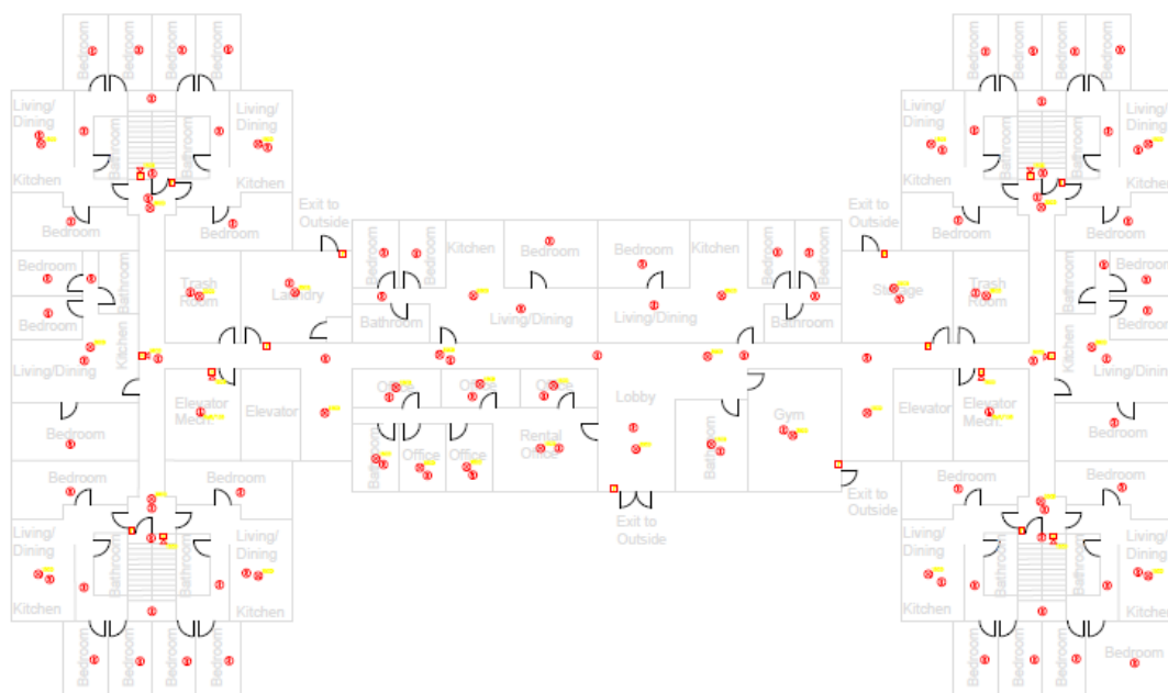
Figure 18: Fire Alarm Design - Case 2, Floor 1
