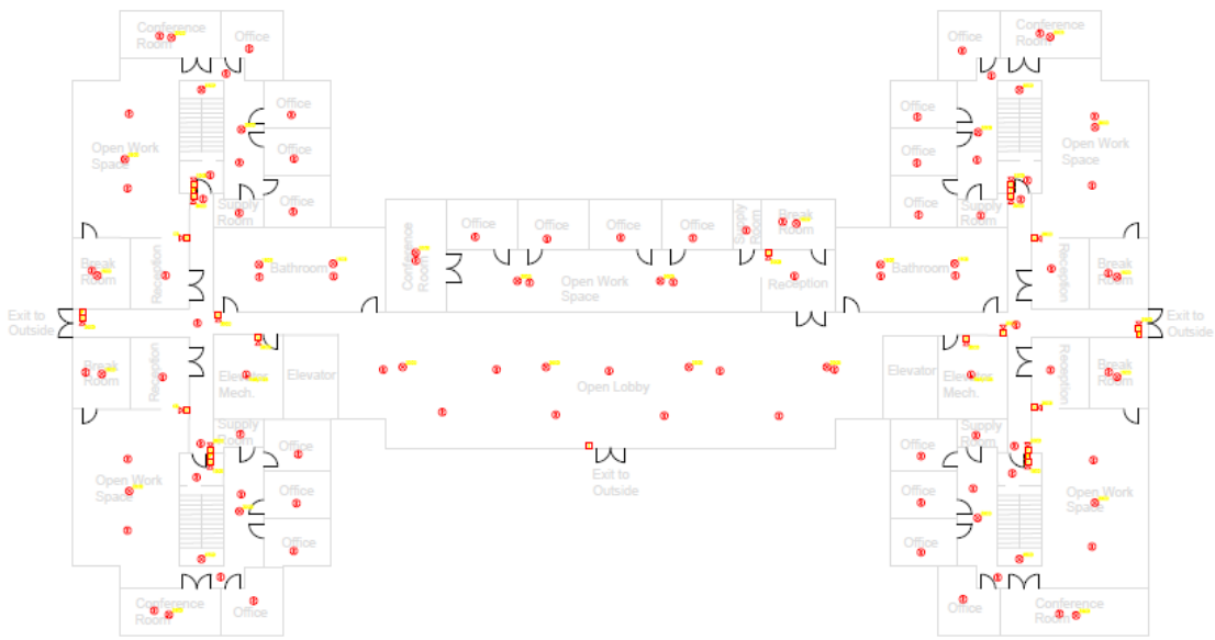
Figure 12: Fire Alarm Design - Case 1, Floor 1
