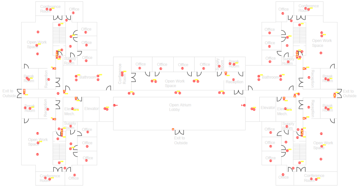
Figure 27: Fire Alarm Design - Case 4, Floor 1
