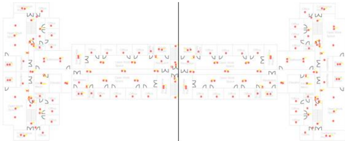
Figure 37: Fire Alarm Design - Case 5, Floors 2-5
