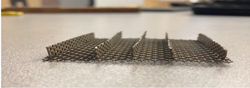
**Figure 8:** Thermal pathing design for a paraffin wax PCM requiring thermal pathing due to low thermal conductivity in the PCM. The bottom mesh is stainless steel while the fins are aluminum.
