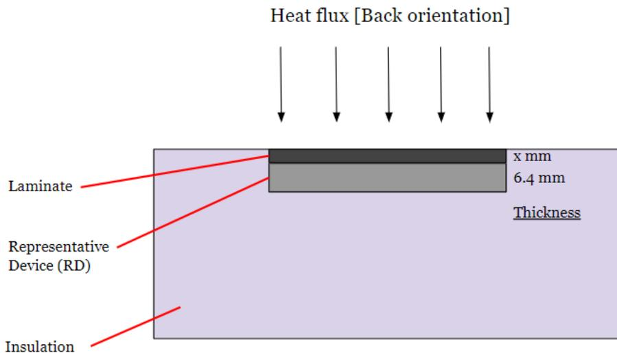
**Figure 48:** The orientation for the laminate tests. For the Nomex laminate,  $x$  is 1.5 mm, while for the AS fiberglass laminate test,  $x$  is 1.6mm. This figure is not made to scale.
