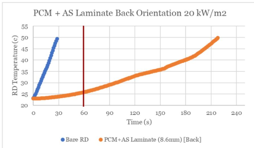
**Figure 36:** This is the data for the representative device temperature vs time with the PCM above the representative device in the front orientation at  $20 \text{ kW/m}^2$ . Above the PCM is the AS fiberglass laminate. The thickness is 8.6 mm because the PCM is 7 mm thick while the AS laminate is 1.6mm thick. Highlighted in red is the success time for this test.
