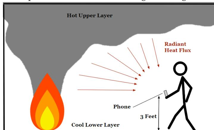
**Figure 2:** A simple diagram showing the approximate position of a phone in a compartment fire. Heat flux is incoming from both the fire itself and the hot smoke above. The backside and screen of the phone are both exposed to fire when the phone is in use.
