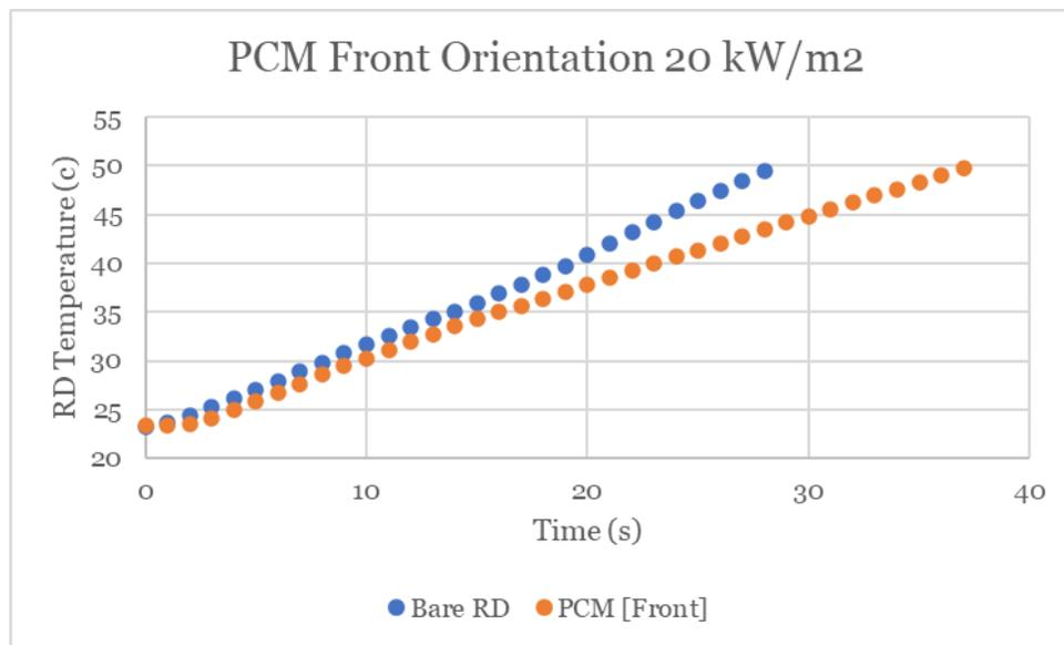
**Figure 30:** This is the data for the representative device temperature vs time with the PCM beneath the representative device in the Front orientation at 20 kW/m<sup>2</sup>.
