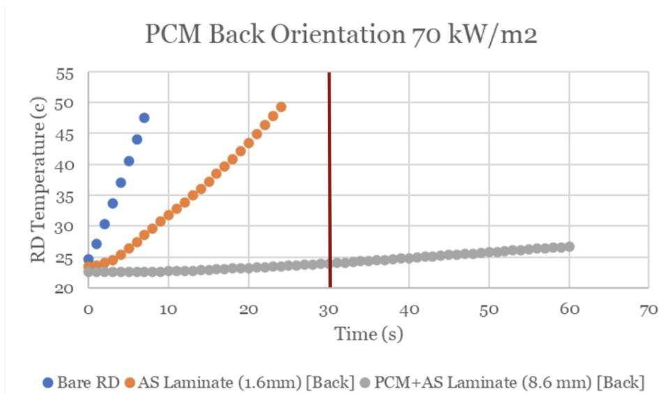
**Figure 68:** The combined data for the bare RD, the AS laminate, and the back orientation PCM tests at 70 kW/m<sup>2</sup>. Highlighted in red is the success time for these tests.
