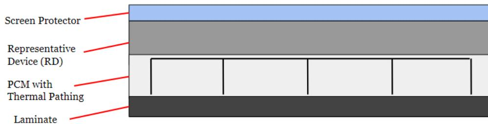
**Figure 12:** General design for the full casing layout. From back to front (bottom to top in this figure), the layout consists of the laminated outer casing, the PCM with thermal pathing, the representative device, and the screen protection glass. This figure is not to scale.
