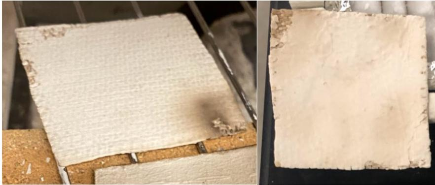
**Figure 37:** Before (left) and after (right) photos of the AS fiberglass laminate following the test with the PCM and the laminate conducted at  $20 \text{ kW/m}^2$ .
