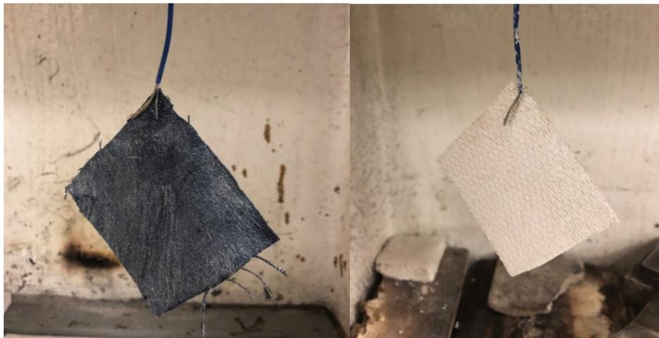
**Figure 73:** Initial coatings on the laminates were allowed to dry shown above. Nomex pictured on the left and the AS Fiberglass on the right.
