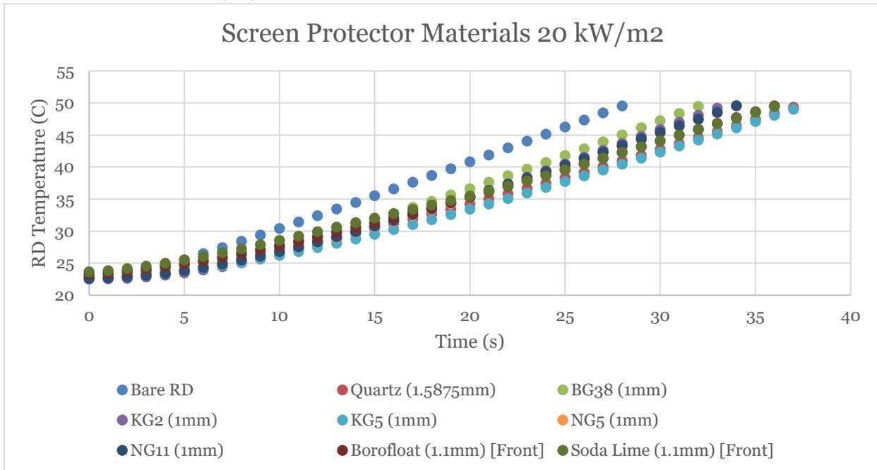
**Figure 72:** The results of testing all screen protector materials, both during the main and follow-up study.
