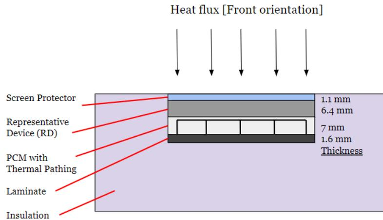
**Figure 14:** This diagram shows an example of a sample setup which will be tested in our experiments. In this layout, the configuration shows the flux directed at the frontside of the casing system, wherein the “screen” faces upwards towards the heat source. This figure is not made to scale. Additionally, it specifies a laminate thickness of 1.6 mm, but two different laminates were tested, one with thickness of 1.6 mm and one with thickness of 1.5 mm.
