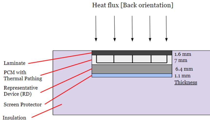
**Figure 15:** This diagram shows an example of a sample setup which will be tested in our experiments. In this layout, the configuration shows the flux directed at the backside of the casing system, wherein the “screen” faces downwards, away from the heat source. This figure is not made to scale. Additionally, it specifies a laminate thickness of 1.6 mm, but two different laminates were tested, one with thickness of 1.6 mm and one with thickness of 1.5 mm.
