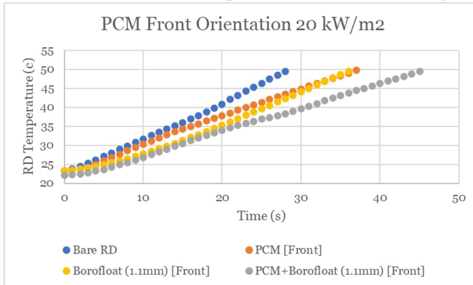
**Figure 62:** The combined data for the bare RD, the Borofloat test, and the front orientation PCM tests at 20 kW/m<sup>2</sup>.
