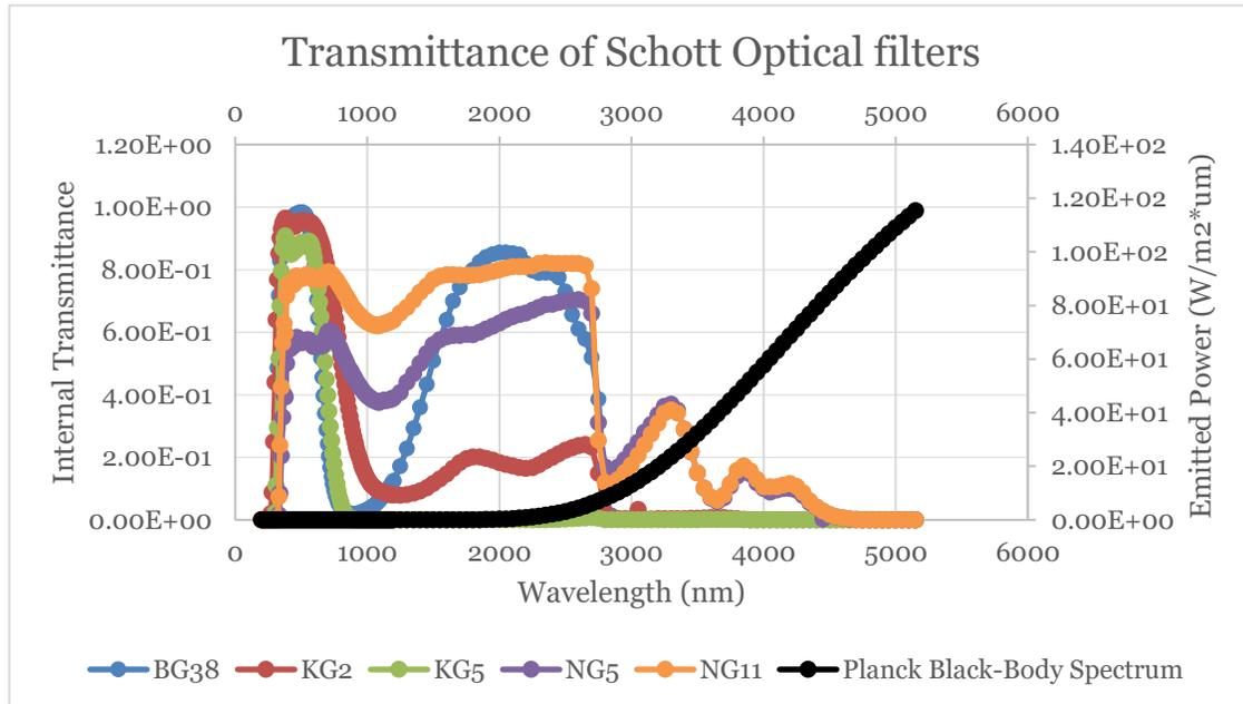
**Figure 6:** The internal transmittance data for the optical filters tested in the follow-up study performed in D-term. The Planck Black-Body Spectrum is plotted on the secondary axis on the right side of the figure for the temperature of 411°C.
