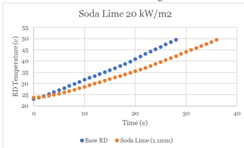
**Figure 20:** This is the data for the representative device temperature vs time with the soda lime glass on top of the representative device to shield it from the heat flux at 20 kW/m<sup>2</sup>.
