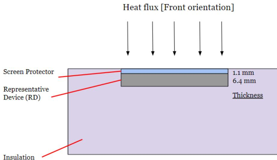
**Figure 18:** The orientation of the setup used for both the Borofloat and the soda lime glass tests. This figure is not made to scale.
