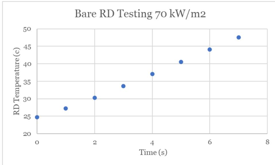
**Figure 39:** This is the data for the representative device temperature vs time without any measures being used to protect it from the heat flux at 70 kW/m<sup>2</sup>.
