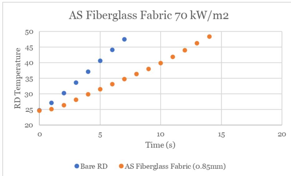
**Figure 47:** This is the data for the representative device temperature vs time with the AS fiberglass fabric on top of the representative device to shield it from the heat flux at  $70 \text{ kW/m}^2$ .
