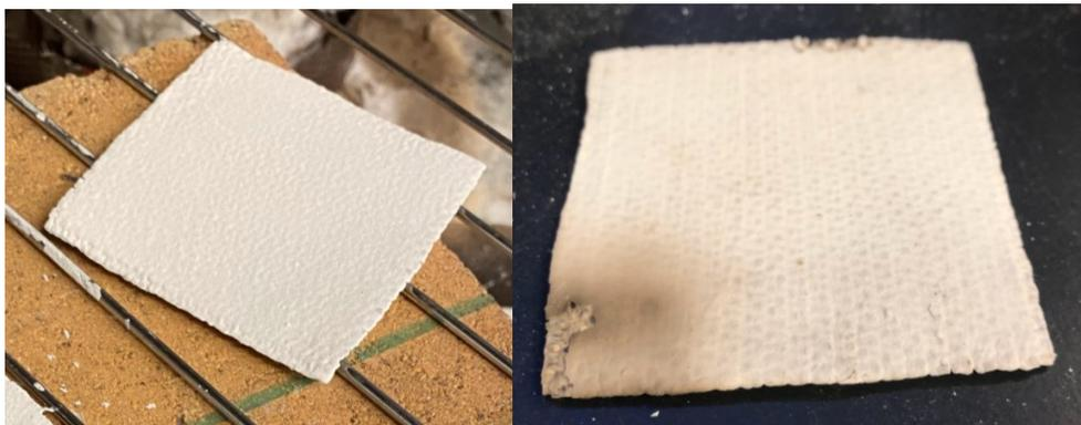
**Figure 52:** Before (left) and after (right) photos of the AS fiberglass laminate following the test with just the laminate conducted at 70 kW/m<sup>2</sup>.
