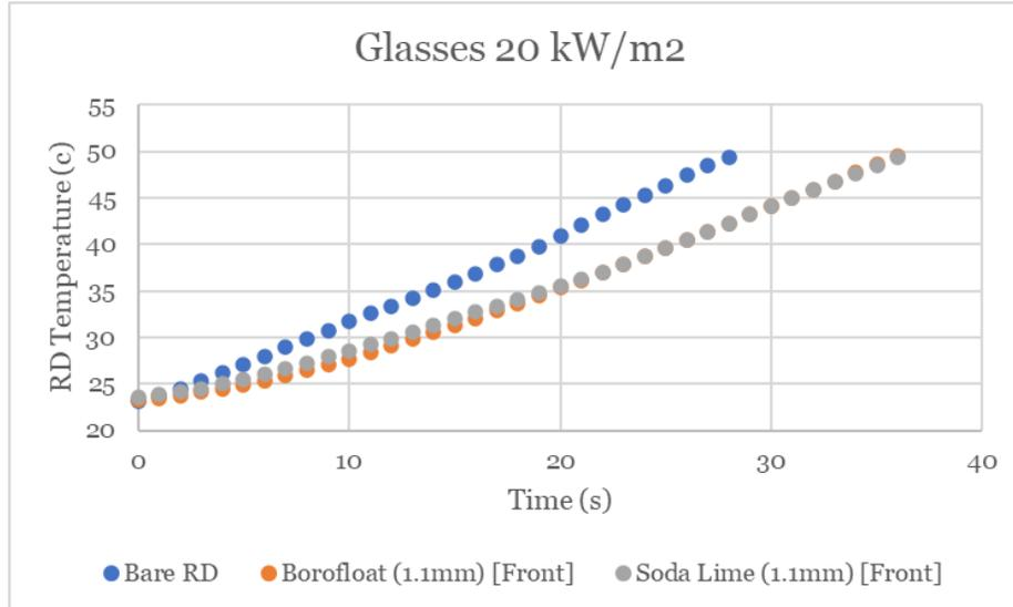
**Figure 59:** The combined data for the bare RD and both glass tests performed at 20 kW/m<sup>2</sup>.
