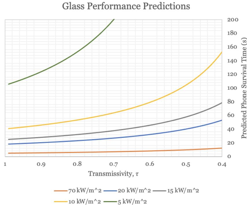
**Figure 70:** This chart shows the predicted time of phone survival when changing the transmissivity of the glass. Each line corresponds to a heat flux that is held constant.
