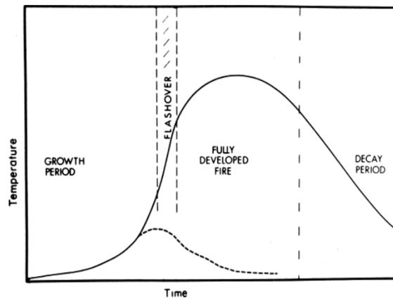
**Figure 1:** The temperature profile over time of a developing compartment fire. Figure is sourced from “Analysis of the compartment fire parameters influencing the heat flux incident on the structural façade” (Abecassis).
