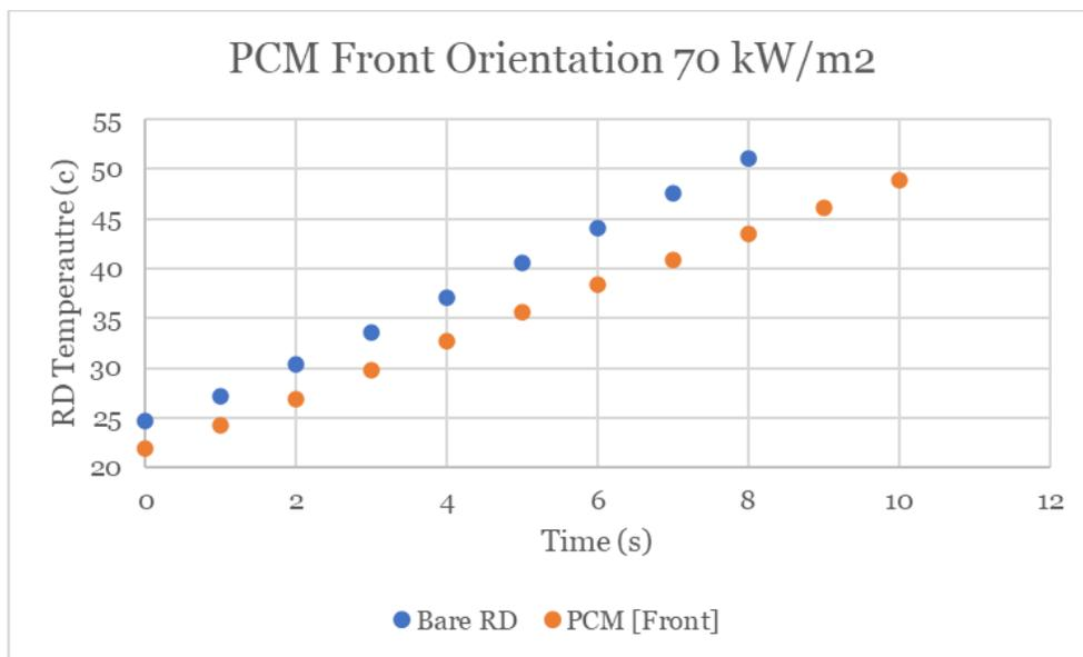
**Figure 54:** This is the data for the representative device temperature vs time with the PCM beneath the representative device in the Front orientation at  $70 \text{ kW/m}^2$ .
