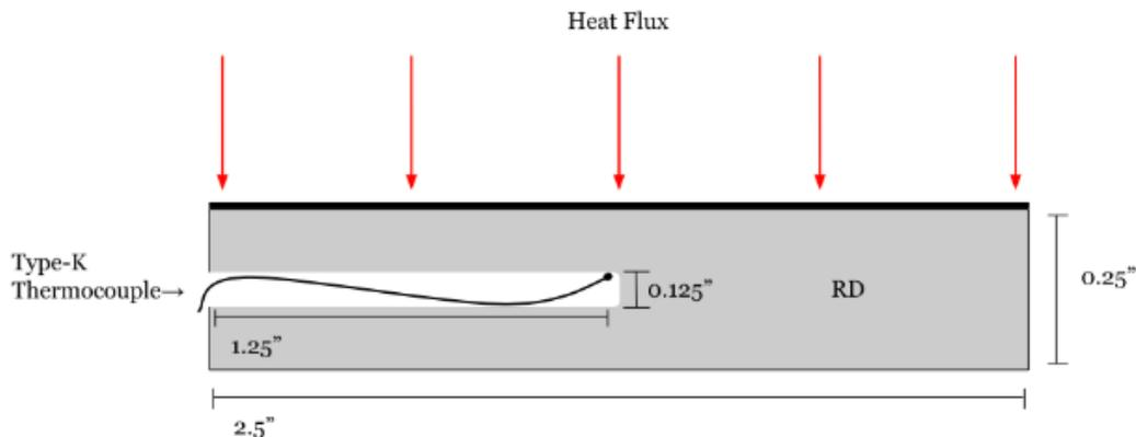
**Figure 13:** Thermocouple orientation within the representative device. Dimensions provided are accurate, but the figure is not to scale.
