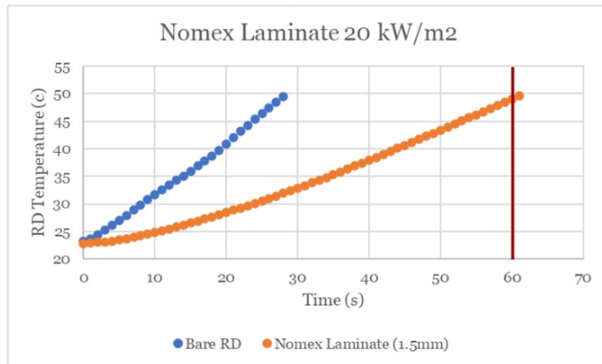
**Figure 27:** This is the data for the representative device temperature vs time with the Nomex laminate on top of the representative device to shield it from the heat flux at 20 kW/m<sup>2</sup>. Highlighted in red is the success time for this test.
