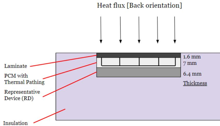
**Figure 35:** The testing setup for the PCM and AS fiberglass laminate test in the back orientation. This figure is not made to scale.
