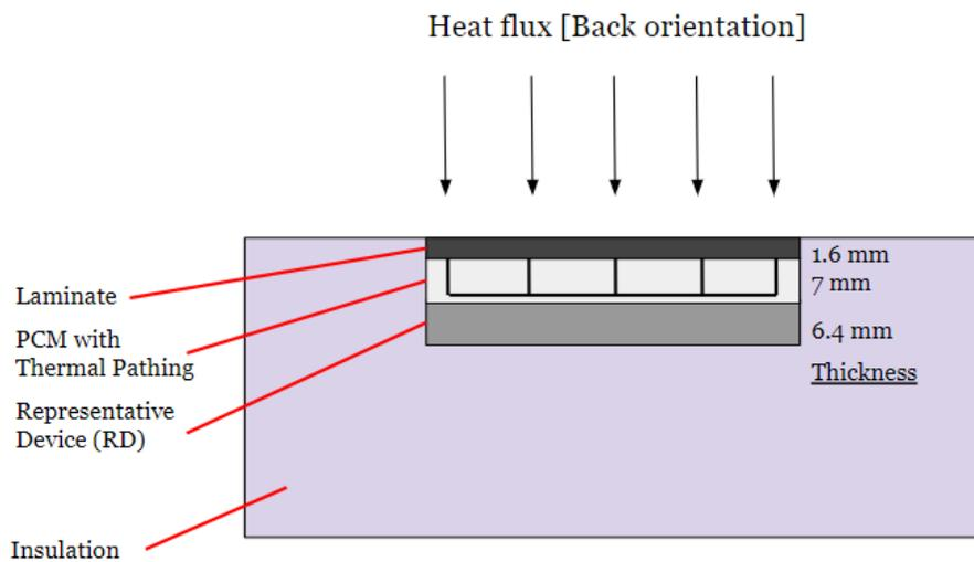
**Figure 56:** The testing setup for the PCM and AS fiberglass laminate test in the back orientation. This figure is not made to scale.
