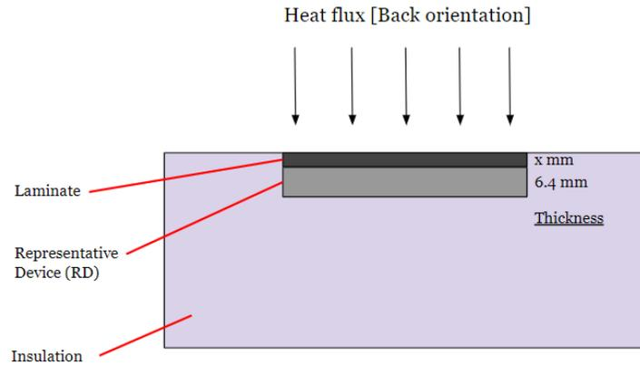
**Figure 26:** The orientation for the laminate tests. For the Nomex laminate,  $x$  is 1.5 mm, while for the AS fiberglass laminate test,  $x$  is 1.6mm. This figure is not made to scale.
