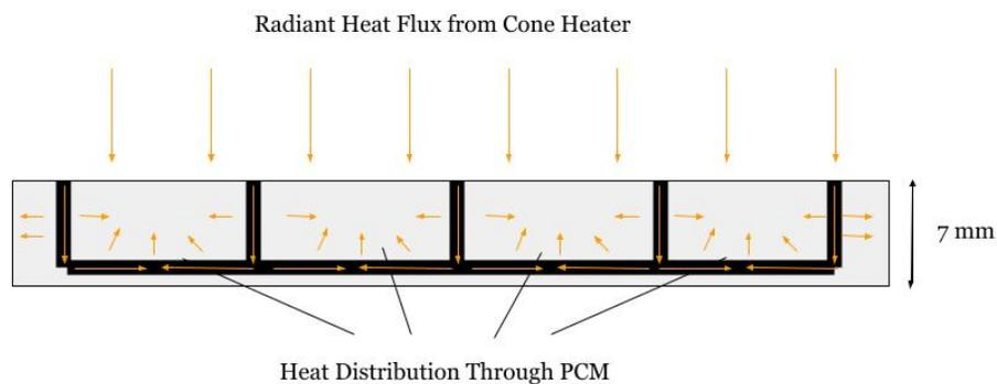
**Figure 10:** Figure showing how heat is distributed through the PCM with the thermal pathing. Without the thermal pathing, heat is only hitting the top of the PCM layer, and is not distributed by the metal of the thermal pathing.
