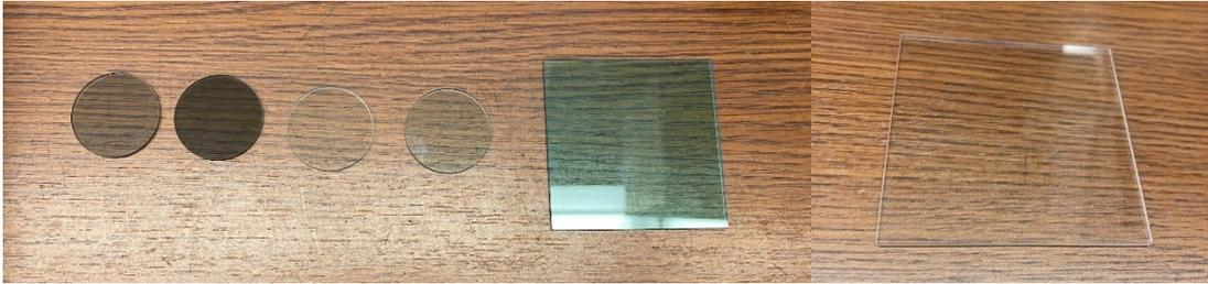
**Figure 5:** The materials used in the follow-up study. From left to right: NG11, NG5, KG2, KG5, BG38, and Quartz high temperature glass.
