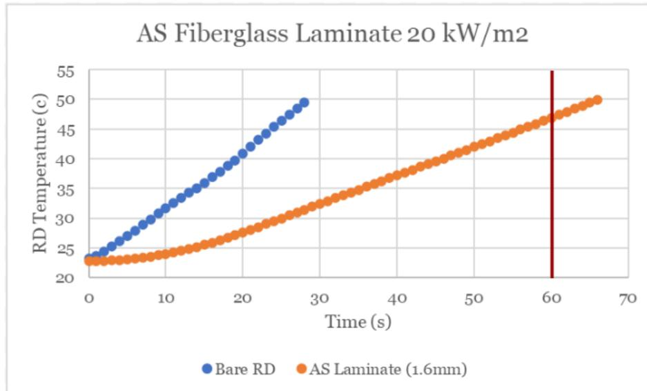
**Figure 28:** This is the data for the representative device temperature vs time with the AS fiberglass laminate on top of the representative device to shield it from the heat flux at 20 kW/m<sup>2</sup>. Highlighted in red is the success time for this test.
