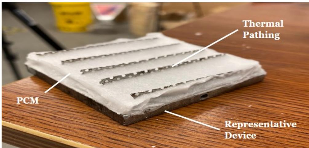
**Figure 9:** Thermal pathing filled with paraffin wax on top of the representative device.
