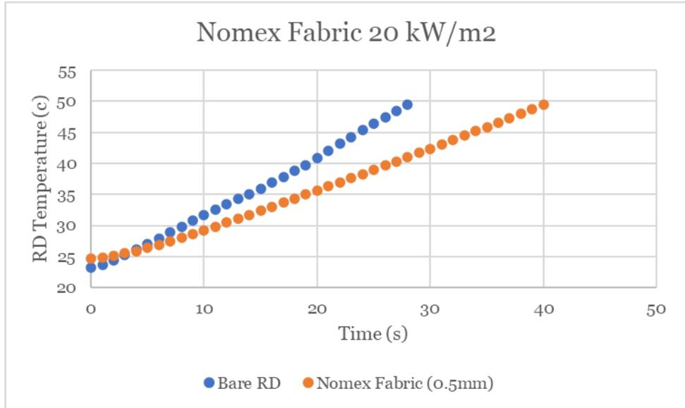
**Figure 22:** This is the data for the representative device temperature vs time with the Nomex fabric on top of the representative device to shield it from the heat flux at 20 kW/m<sup>2</sup>.
