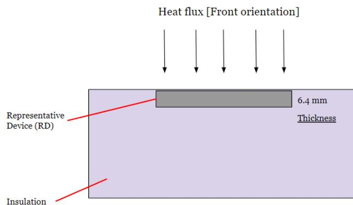
**Figure 38:** The testing setup used for the bare representative device test. This figure is not made to scale.
