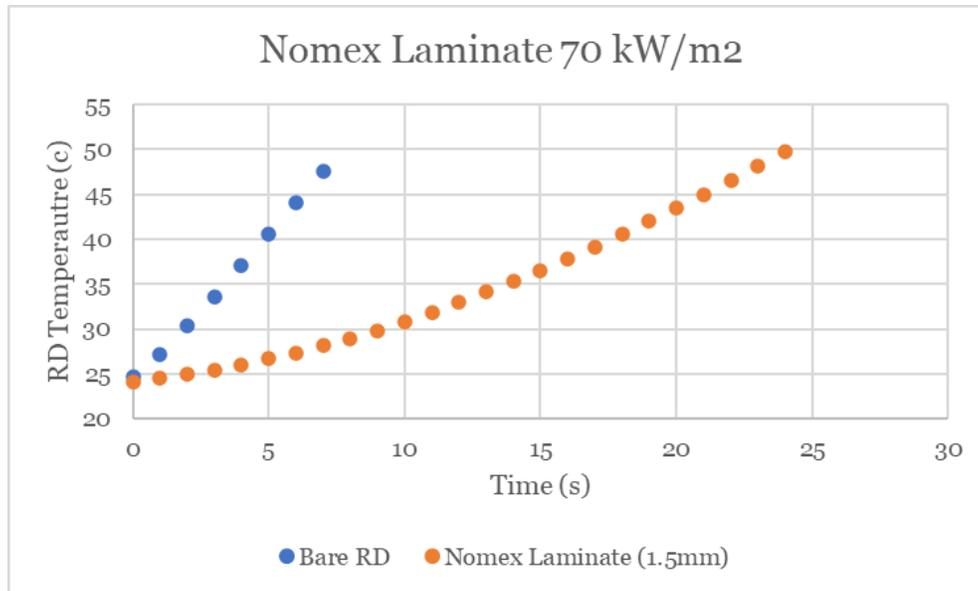
**Figure 49:** This is the data for the representative device temperature vs time with the Nomex laminate on top of the representative device to shield it from the heat flux at 70 kW/m<sup>2</sup>.
