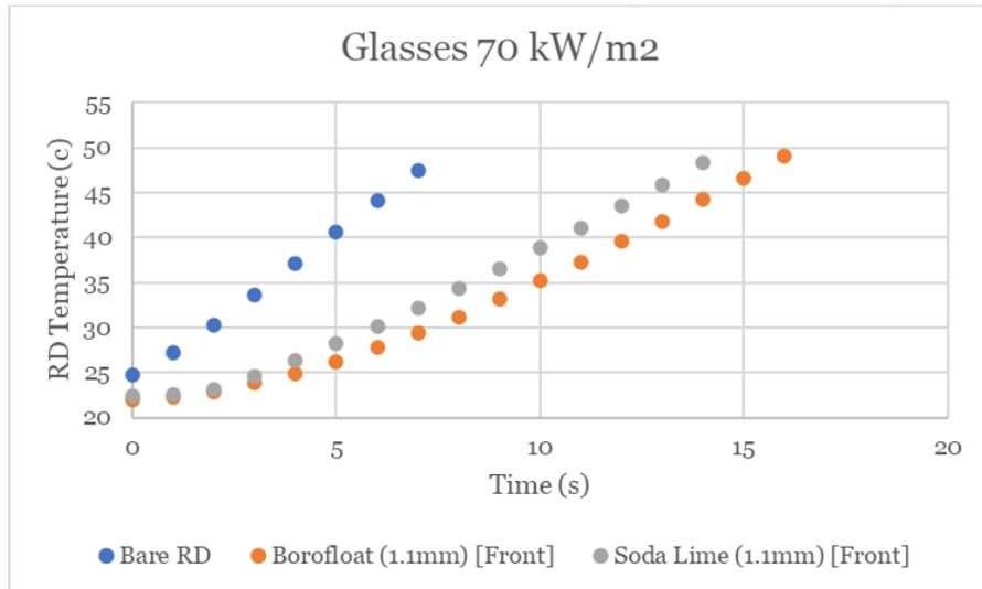
**Figure 65:** The combined data for the bare RD and both glass tests performed at 70 kW/m<sup>2</sup>.
