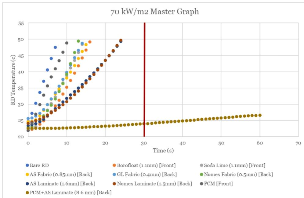
**Figure 69:** The combined data for all the tests conducted at 70 kW/m<sup>2</sup>. Highlighted in red is the success time for these tests.
