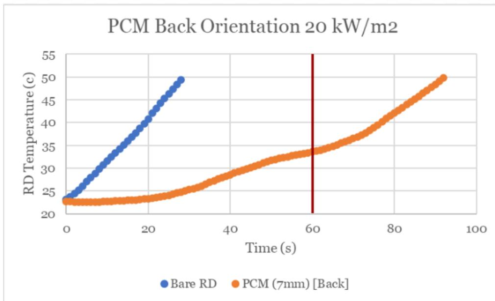
**Figure 32:** This is the data for the representative device temperature vs time with the PCM above the representative device in the back orientation at 20 kW/m<sup>2</sup>. Highlighted in red is the success time for this test.
