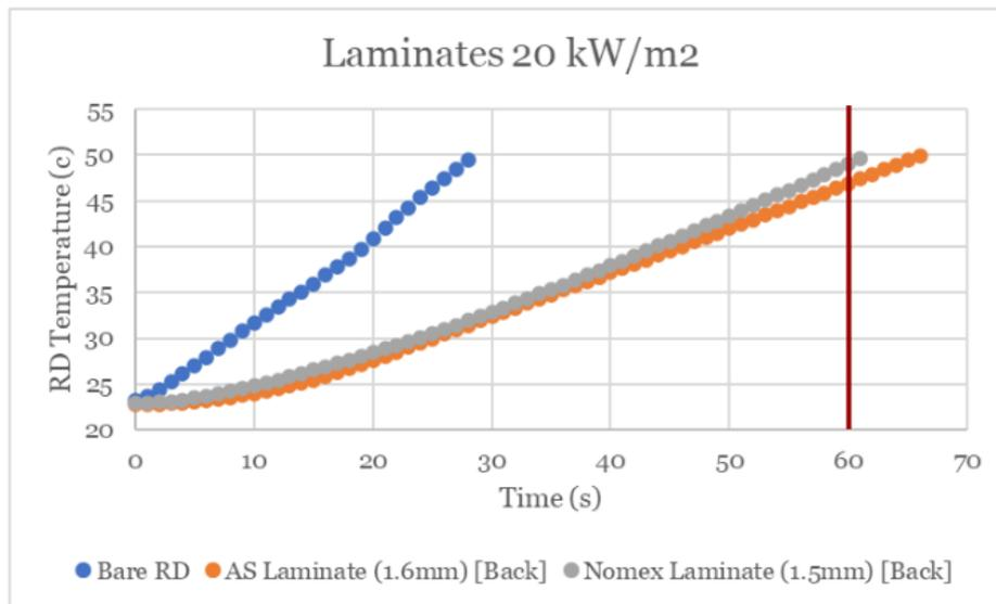
**Figure 61:** The combined data for the bare RD and the laminate tests at 20 kW/m<sup>2</sup>. Highlighted in red is the success time for these tests.
