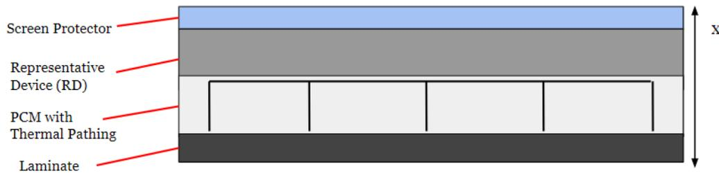
**Figure 3:** This diagram shows a simplified version of the 1-Dimensional system which will be considered for this analysis. In this investigation, heat flux will be considered along the “*x-direction*” as labeled. This figure is not to scale.
