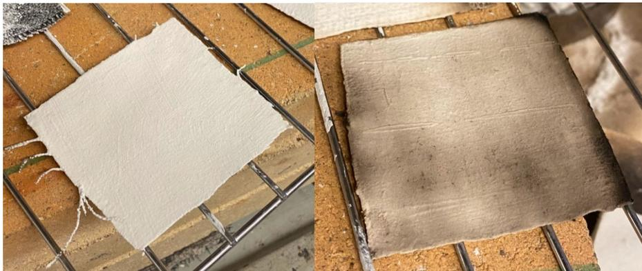
**Figure 50:** Before (left) and after (right) photos of the Nomex laminate following the test conducted at 70 kW/m<sup>2</sup>.
