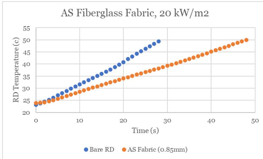
**Figure 24:** This is the data for the representative device temperature vs time with the AS fiberglass fabric on top of the representative device to shield it from the heat flux at 20 kW/m<sup>2</sup>.
