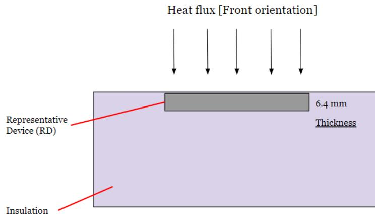
**Figure 16:** The testing setup used for the bare representative device test. This figure is not made to scale.
