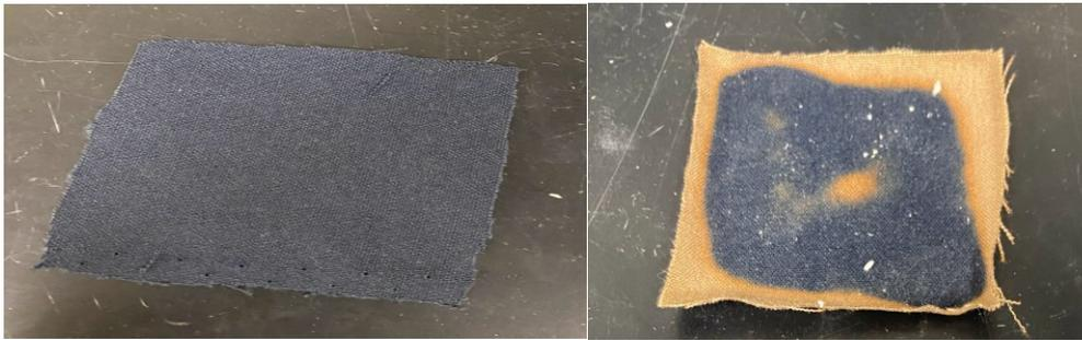
**Figure 23:** Before (left) and after (right) photos of the Nomex fabric following the test conducted at 20 kW/m<sup>2</sup>.
