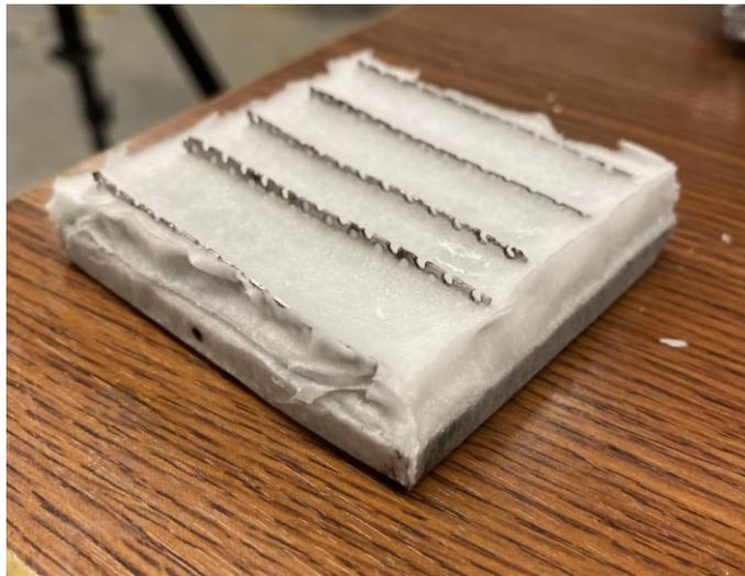
**Figure 76:** This image shows the PCM when fully solidified. The solid PCM surrounds the thermal pathing, and the RD sits underneath it.
