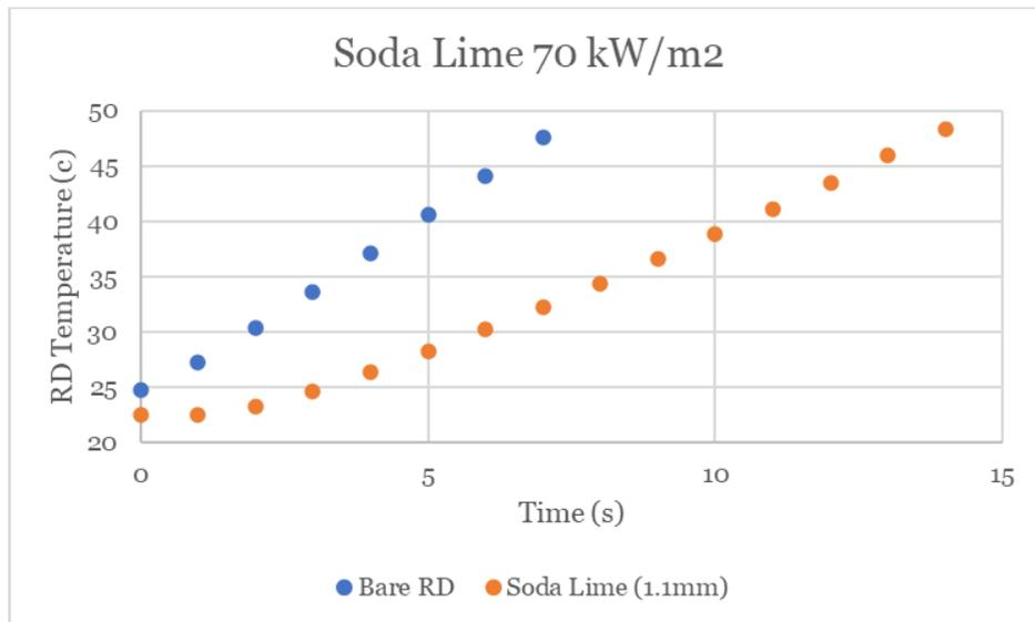
**Figure 42:** This is the data for the representative device temperature vs time with the soda lime glass on top of the representative device to shield it from the heat flux at 70 kW/m<sup>2</sup>.
