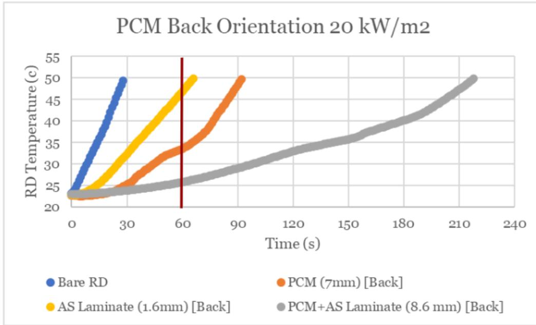
**Figure 63:** The combined data for the bare RD, the AS laminate, and the back orientation PCM tests at 20 kW/m<sup>2</sup>. Highlighted in red is the success time for these tests.
