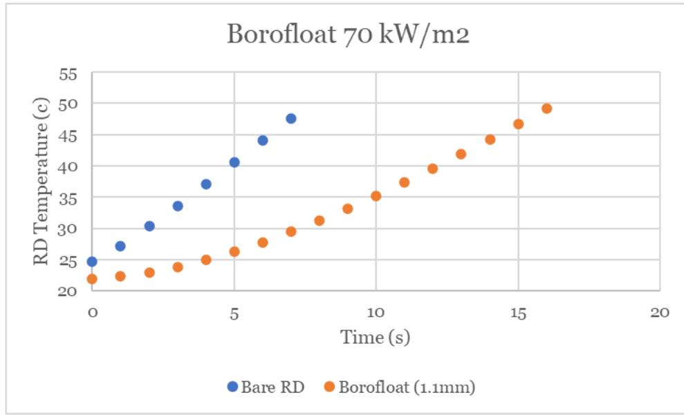
**Figure 41:** This is the data for the representative device temperature vs time with the Borofloat glass on top of the representative device to shield it from the heat flux at 70 kW/m<sup>2</sup>.
