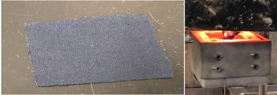
**Figure 45:** The Nomex fabric before the 70 kW/m<sup>2</sup> test and while it was allowed to burn out under the cone heater.
