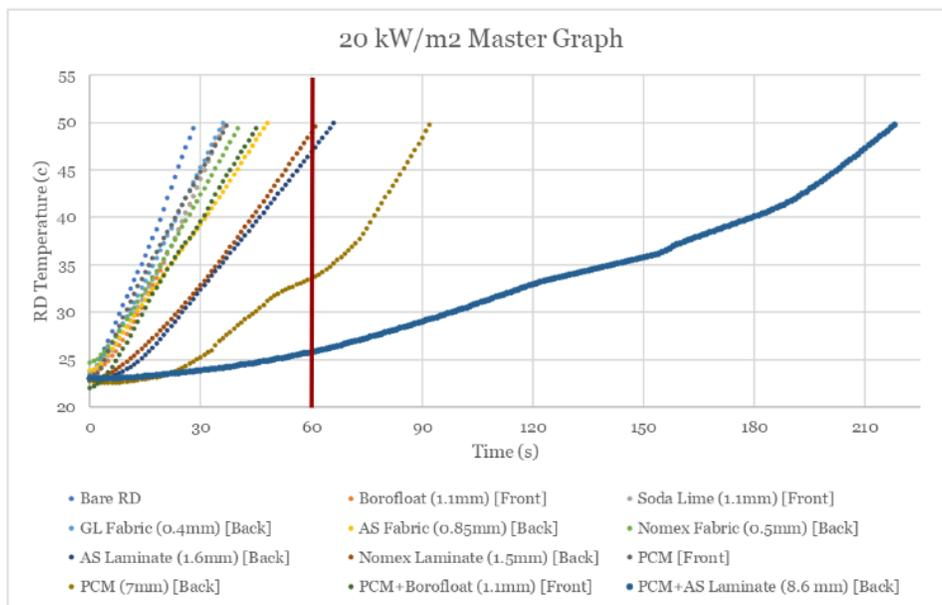
**Figure 64:** The combined data for all the tests conducted at 20 kW/m<sup>2</sup>. Highlighted in red is the success time for these tests.
