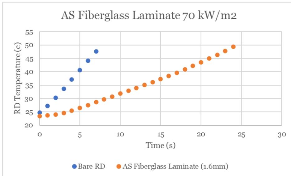
**Figure 51:** This is the data for the representative device temperature vs time with the AS fiberglass laminate on top of the representative device to shield it from the heat flux at 70 kW/m<sup>2</sup>.
