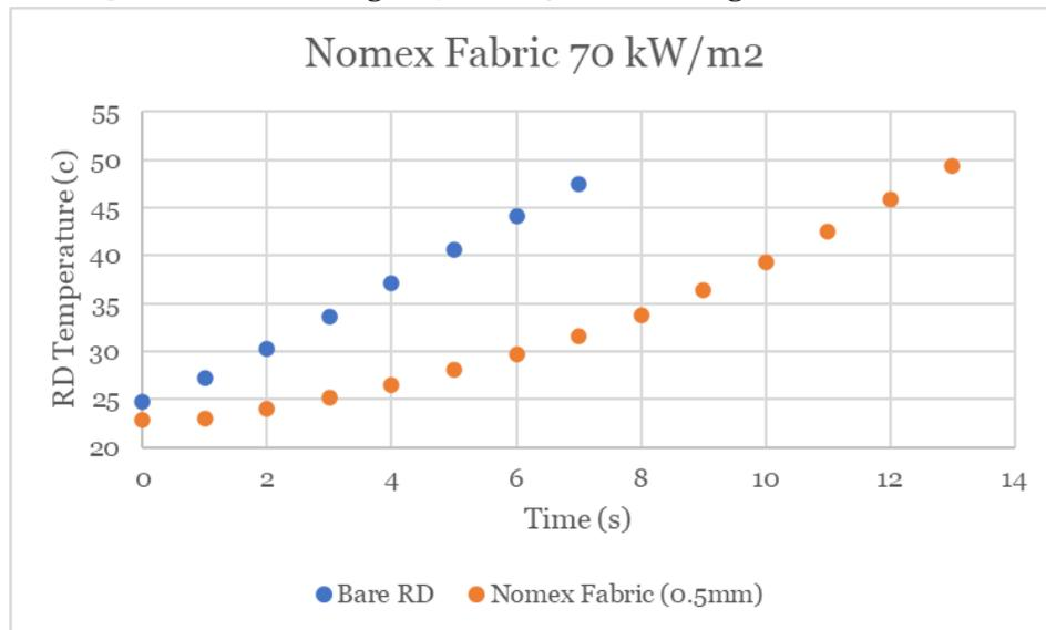
**Figure 44:** This is the data for the representative device temperature vs time with the Nomex Fabric on top of the representative device to shield it from the heat flux at 70 kW/m<sup>2</sup>.
