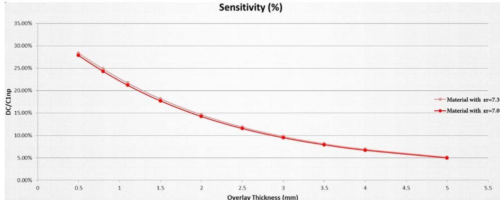
**Figure 4:** Sensitivity of a touch screen compared to the thickness of the overlay material and the permittivity of the material. The x-axis is the thickness of the material, while the y-axis is the sensitivity of the screen. The two separate lines are tests for two separate materials, with slight differences in their permittivity. Figure is sourced from “Touch Sensor Front Panel: How to Choose the Right Cover Glass” (Fieldscale).
