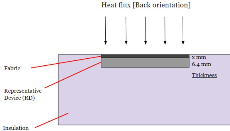
**Figure 21:** The test setup orientation for the fabric tests. For the Nomex, the thickness,  $x$ , is 0.5 mm. For the AS fiberglass, the thickness,  $x$ , is 0.85. For the GL fiberglass,  $x$  is 0.4 mm. This figure is not made to scale.
