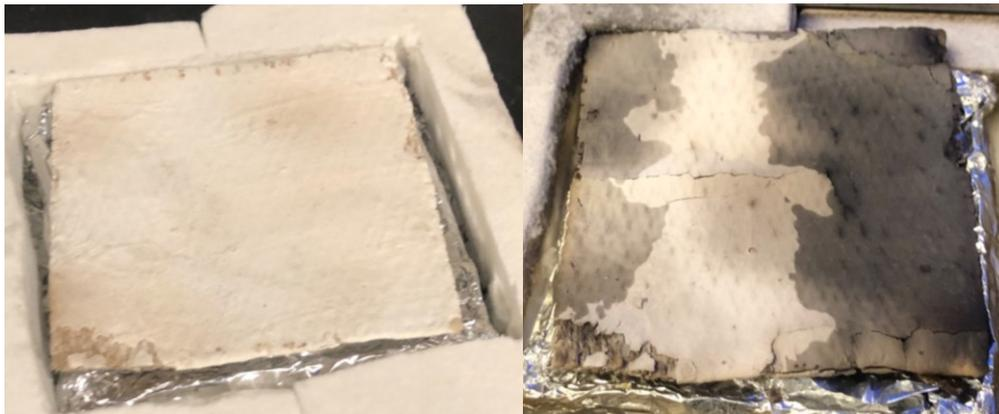
**Figure 58:** Before (left) and after (right) photos of the AS fiberglass laminate following the test conducted with the PCM and the laminate at 70 kW/m<sup>2</sup>.
