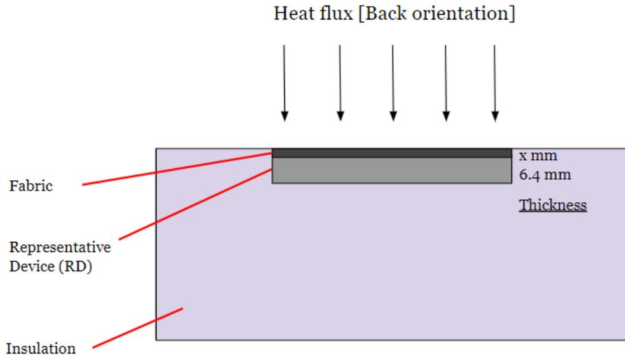
**Figure 43:** The test setup orientation for the fabric tests. For the Nomex, x is 0.5 mm. For the AS fiberglass, x is 0.85. For the GL fiberglass, x is 0.4 mm. This figure is not made to scale.
