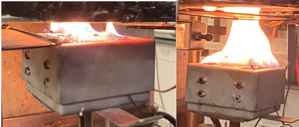
**Figure 55:** The PCM fire that occurred while doing the front orientation PCM test at  $70 \text{ kW/m}^2$ .
