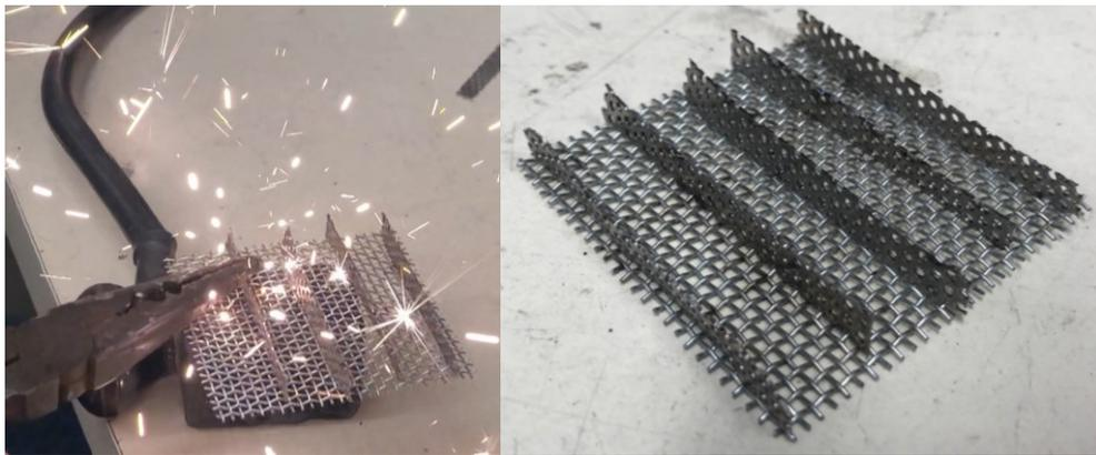
**Figure 74:** These two images taken in the lab show the spot welding of the fins (left) and the finished thermal pathing network (right).
