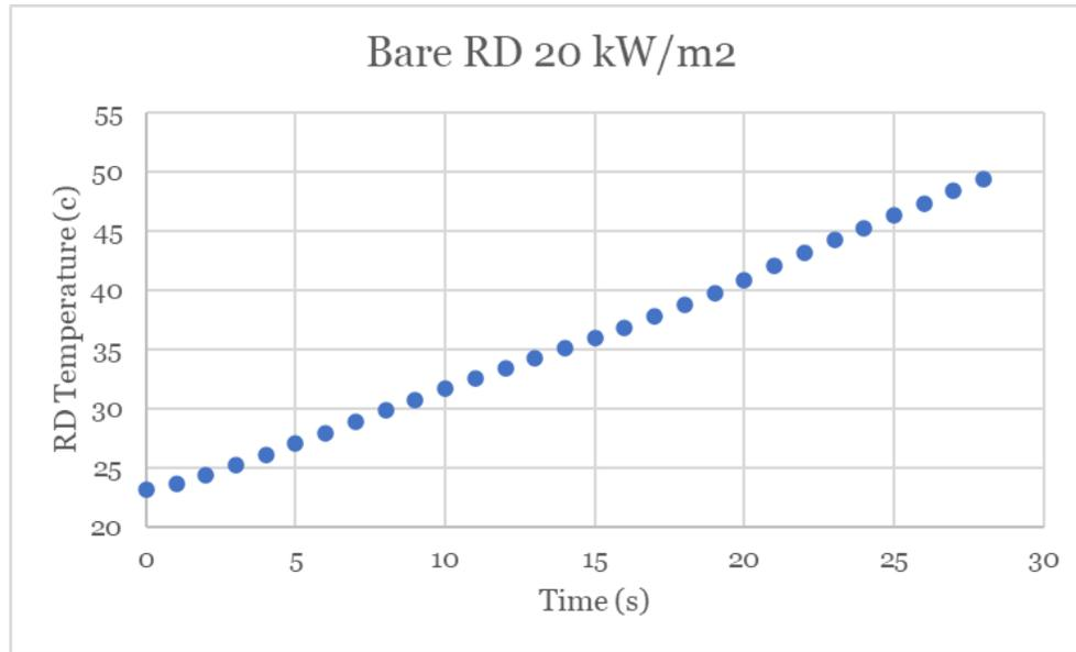
**Figure 17:** This is the data for the representative device temperature vs time without any measures being used to protect it from the heat flux at 20 kW/m<sup>2</sup>.
