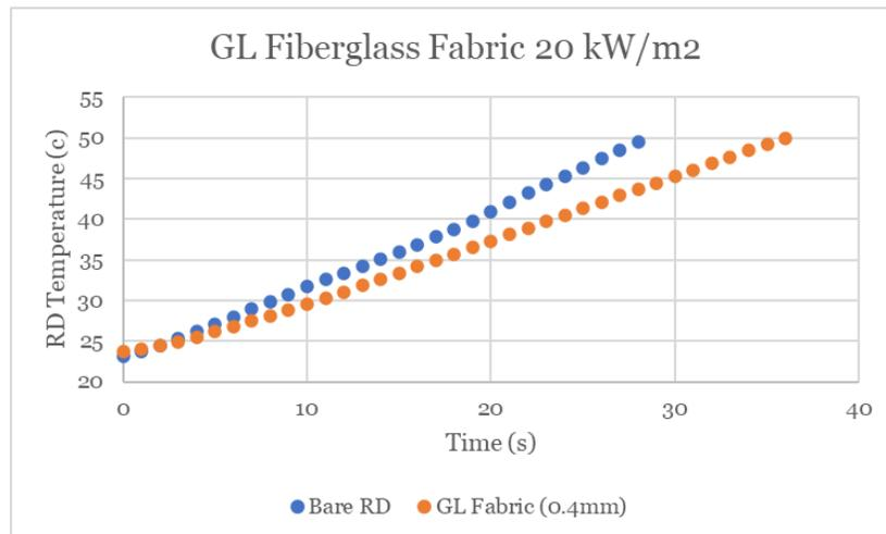
**Figure 25:** This is the data for the representative device temperature vs time with the GL fiberglass fabric on top of the representative device to shield it from the heat flux at 20 kW/m<sup>2</sup>.
