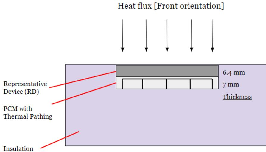
**Figure 29:** The testing setup for the PCM only test in the front orientation. This figure is not made to scale.
