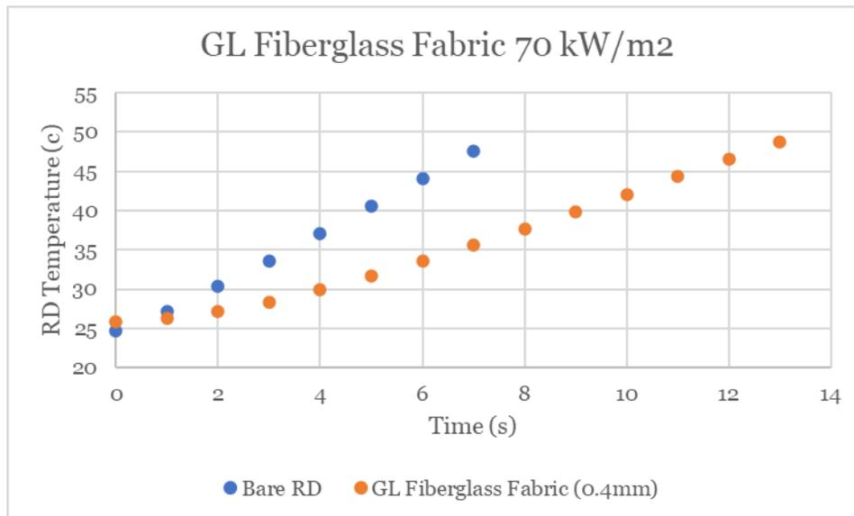
**Figure 46:** This is the data for the representative device temperature vs time with the GL fiberglass fabric on top of the representative device to shield it from the heat flux at 70 kW/m<sup>2</sup>.
