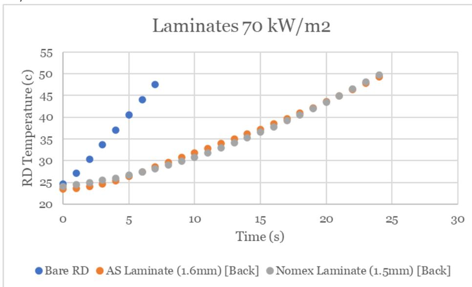
**Figure 67:** The combined data for the bare RD and the laminate tests at 70 kW/m<sup>2</sup>.
