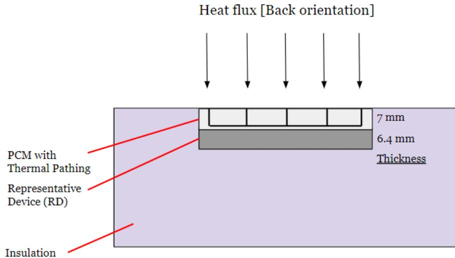
**Figure 31:** The testing setup for the PCM only test in the back orientation. This figure is not made to scale.
