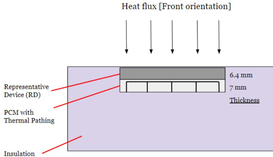
**Figure 53:** The testing setup for the PCM only test in the front orientation. This figure is not made to scale.
