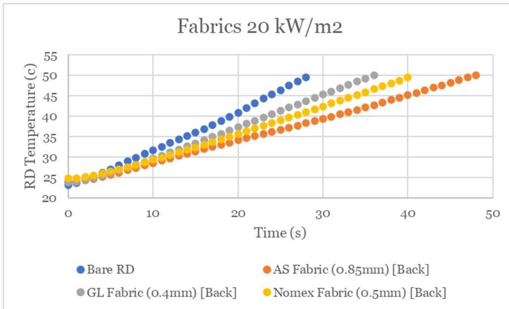
**Figure 60:** The combined data for the bare RD and the fabric tests at 20 kW/m<sup>2</sup>.
