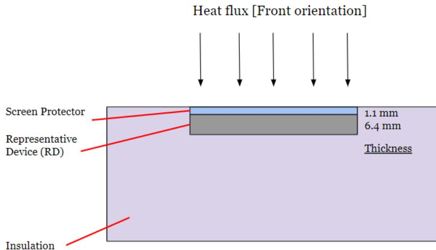
**Figure 40:** The orientation of the setup used for both the Borofloat and the soda lime glass tests. This figure is not made to scale.
