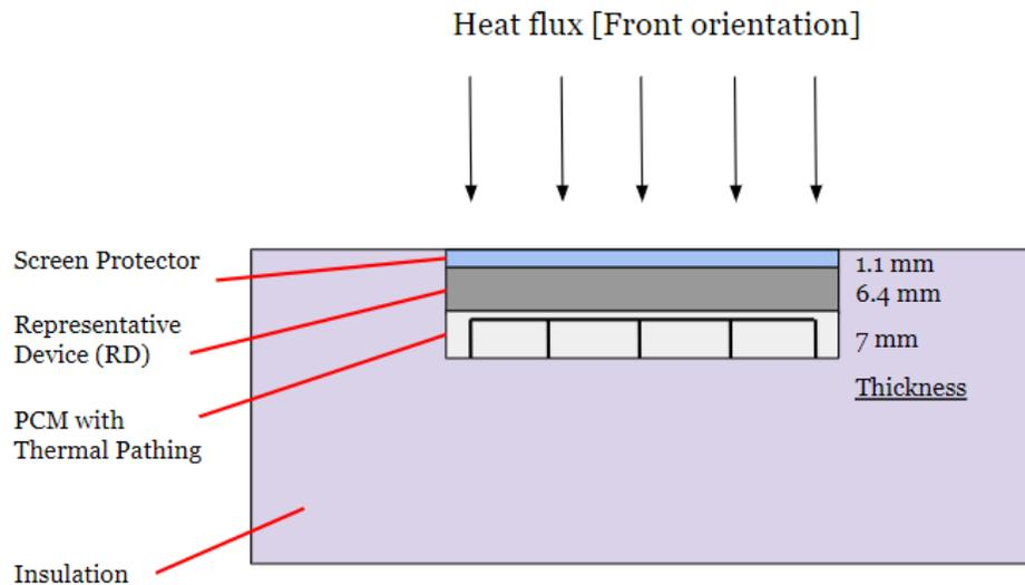
**Figure 33:** The testing setup for the PCM and Borofloat test in the front orientation. This figure is not made to scale.
