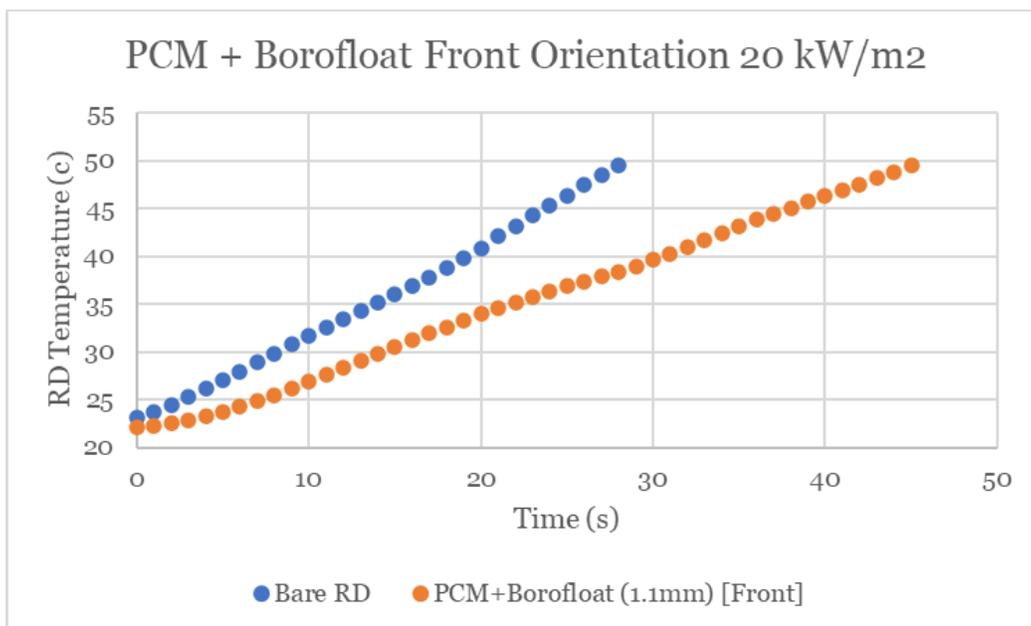
**Figure 34:** This is the data for the representative device temperature vs time with the PCM beneath the representative device and the glass above the representative device in the front orientation at 20 kW/m<sup>2</sup>. Only the glass thickness is considered as the PCM is beneath the representative device.
