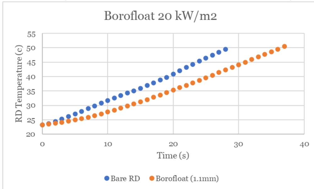
**Figure 19:** This is the data for the representative device temperature vs time with the Borofloat glass on top of the representative device to shield it from the heat flux at 20 kW/m<sup>2</sup>.
