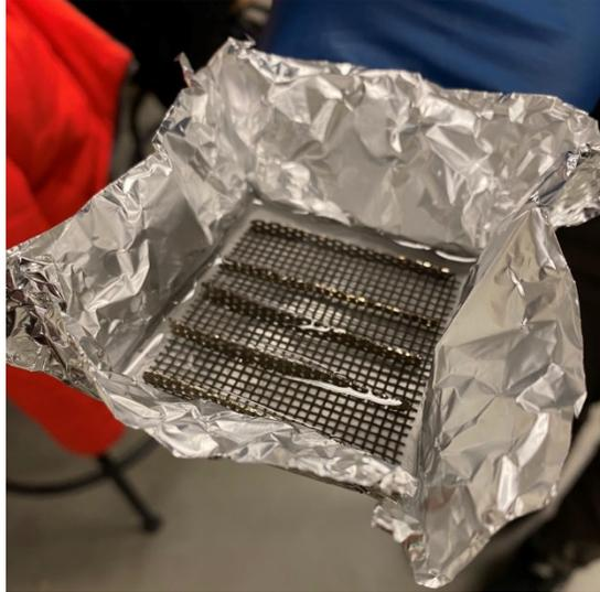
**Figure 75:** This image shows the aluminum mold that was used to contain the liquid PCM when forming. The PCM sits on the back face of the phone where the thermal pathing is submerged.
