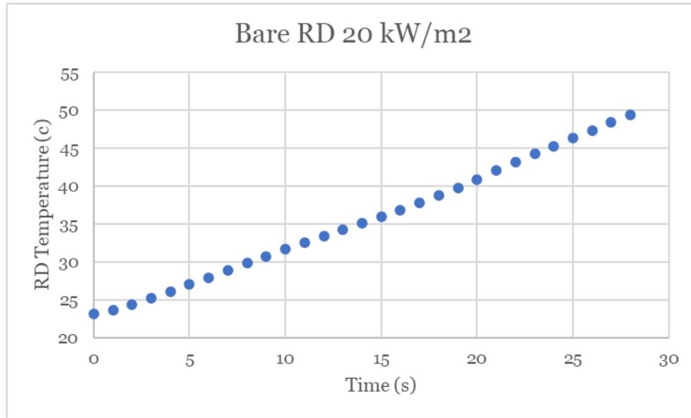
**Figure 17:** This is the data for the representative device temperature vs time without any measures being used to protect it from the heat flux at  $20 \text{ kW/m}^2$ .
