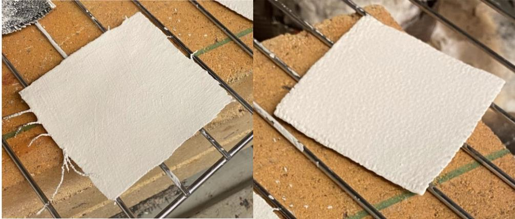
**Figure 11:** The Nomex laminate (left) and the AS fiberglass laminate (right) prior to testing.
