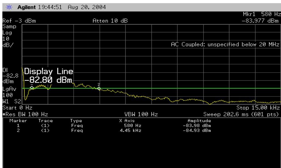
Figure 8-2: Frequency response showing the 10dB bandwidth for ICOM 2TH radio.
