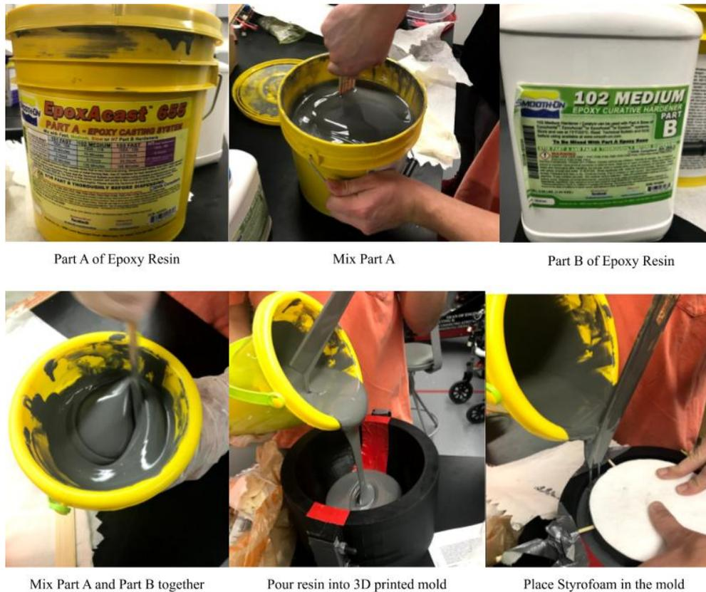
*Figure 6: Top Skull Epoxy Molding Process*
