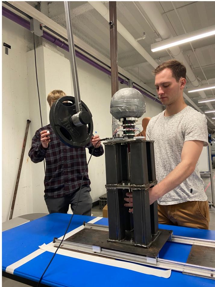
*Figure 17: Fixture and Pendulum Experimental Set-Up*
