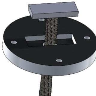
*Figure 10: Original Steel Cable Rotation Prevention Design*
