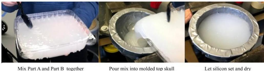
Figure 8: Brain Molding Process
