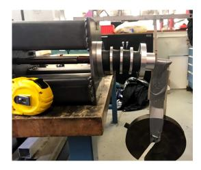
Figure 15: Static Neck Testing Set-Up
