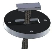
Figure 10: Original Steel Cable Rotation Prevention Design
