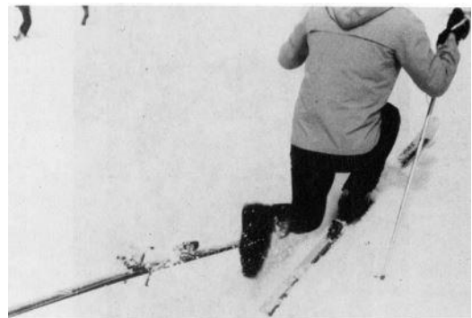
Figure 43: "Bow Effect" Inadvertent Release (Brown and Ettliger, 1985)
