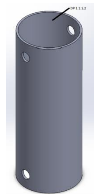
Figure 11: DP 1.1.1.2 Cylindrical Torque Applicator
