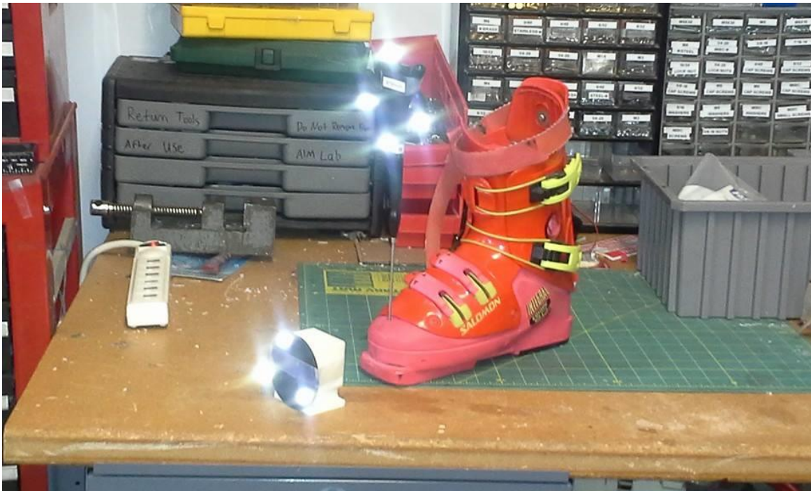
Figure 57: Ski boot with attached passive marker and passive marker reference marker on testing bench
