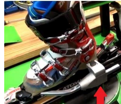
Figure 7: Heel Release Caused by Vertical Force at the Heel (Ski Gear, 2012)
