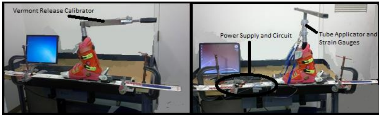
Figure 37: Ski Boot Binding Testing Setup for the Vermont Release Calibrator (left) and the designed device (right)
