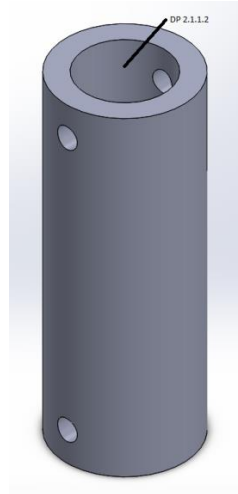
Figure 18: DP 2.1.1.2 Cylindrical torque applicator
