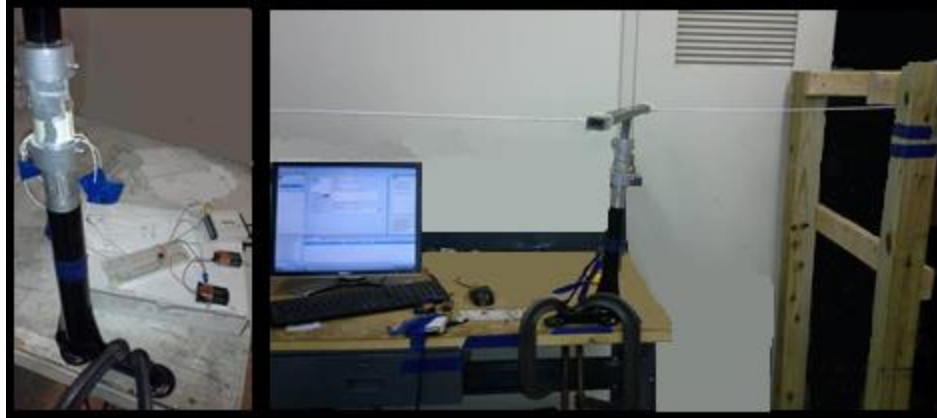
Figure 9: Torque tester in Bending Configuration (Left) and in Twist Configuration (Right)
